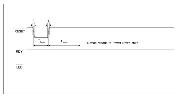
Figure 12.6: Reset Operation
