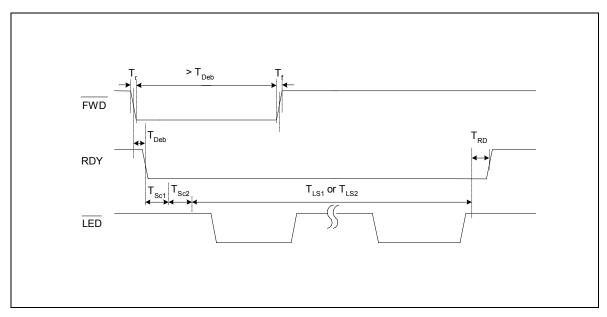
Figure 12.4: Forward Operation with No Sound Effect
