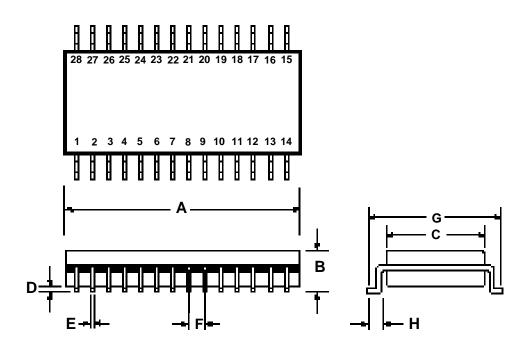
Plastic Small Outline Integrated Circuit (SOIC) Dimensions
