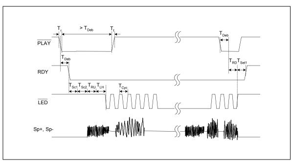
Figure 12.2: Start and Stop Playback Operation
