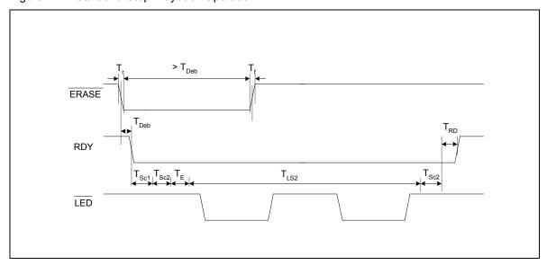
Figure 12.3: Single Erase Operation with No Sound Effect
