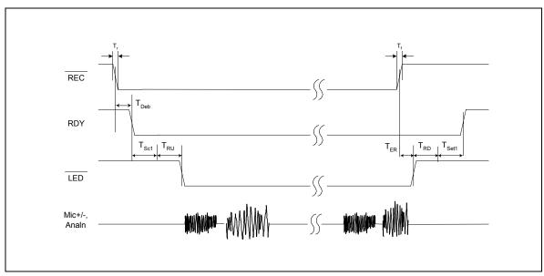
Figure 12.1: Record Operation with No Sound Effect
