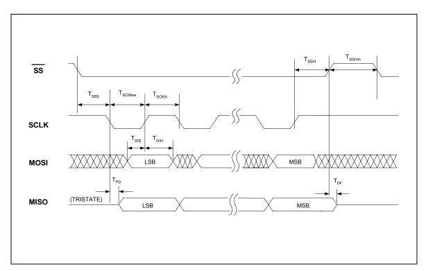
Figure 12.8: SPI Operation
