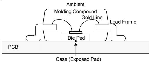
Figure 8. SOP-8 (Exposed Pad) Package Sectional Drawing
