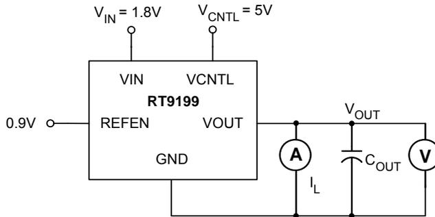
Figure 3. Current Limit for High Side,  $I_{LIM}$
