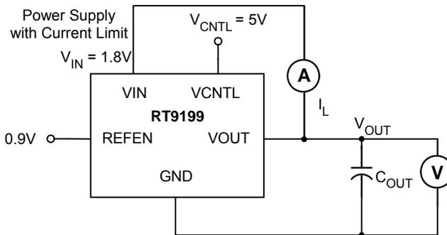
Figure 4. Current Limit for Low Side,  $I_{LIM}$
