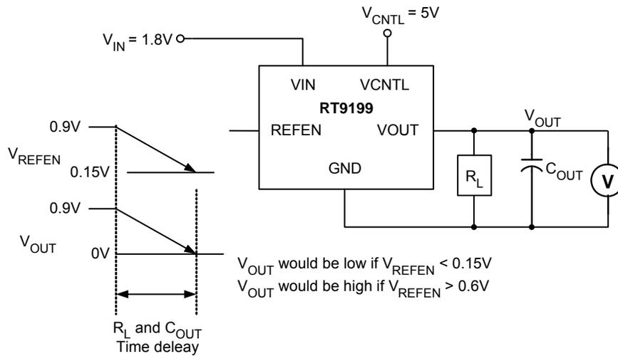
Figure 5. REFEN Pin Shutdown Threshold,  $V_{IH}$  &  $V_{IL}$
