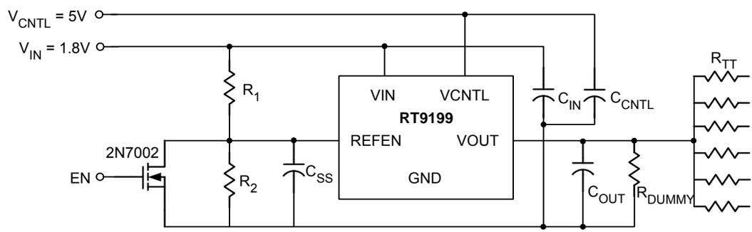
$R_1 = R_2 = 100k\Omega$ ,  $R_{TT} = 50\Omega / 33\Omega / 25\Omega$
