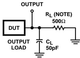
NOTE: For AC Series Only: When  $V_{CC} = 1.5V$ ,  $R_L = 1k\Omega$ .
