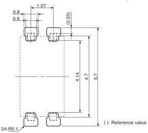
**Remark:** This drawing is considered to meet air and outer creepage distance 4.0 mm minimum. All dimensions in this figure must be evaluated before use.
