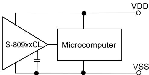
Figure 27 Example for Reset Circuits(S-809xxCL)
