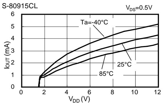
**9. Minimum Operating Voltage - Input Voltage ( $V_{DD}$ )**
