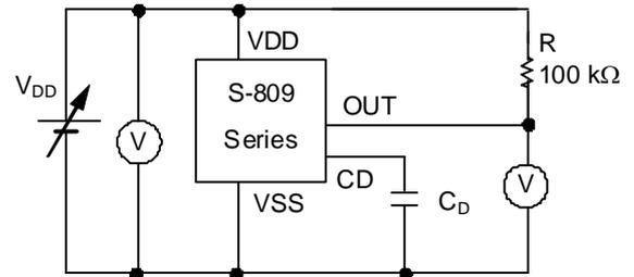
Figure 26 Measurement Circuit for Delay Time
