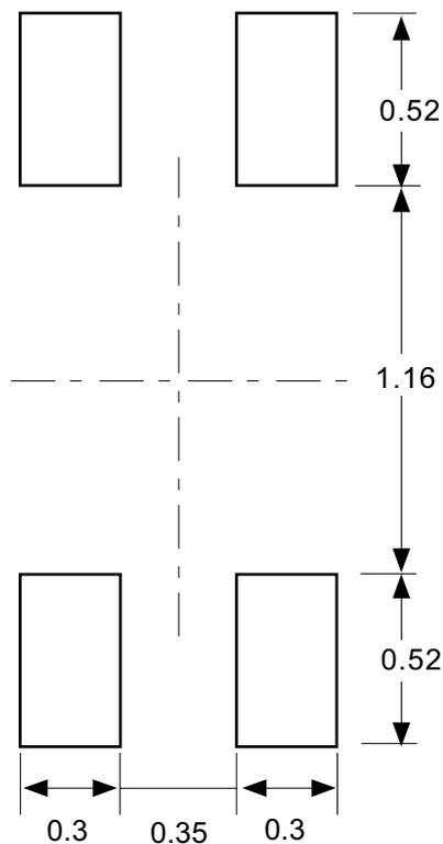
Caution Making the wire pattern under the package is possible. However, note that the package may be upraised due to the thickness made by the silk screen printing and of a solder resist on the pattern because this package does not have the standoff.
