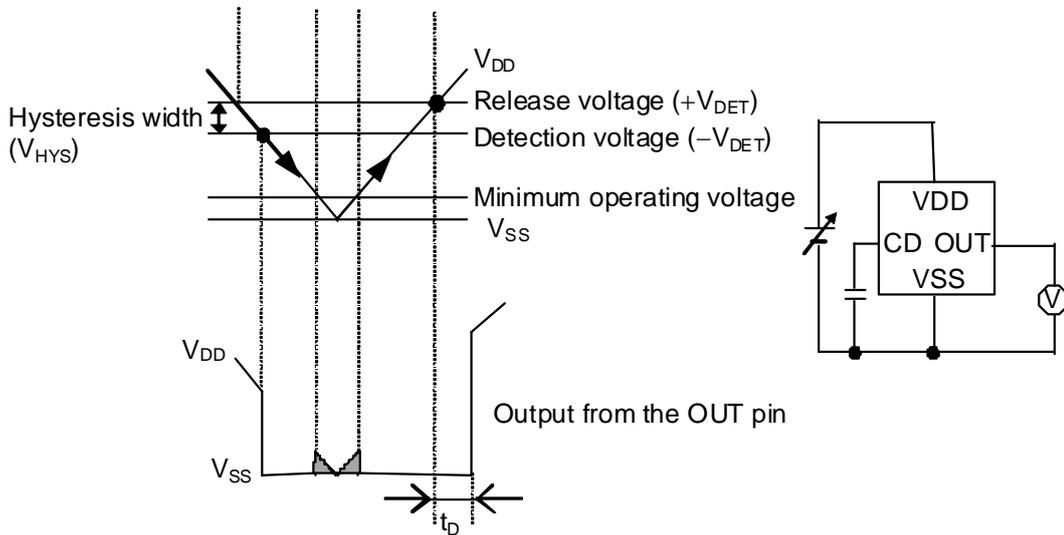
**Remark** For values of  $V_{DD}$  less than minimum operating voltage, values of OUT pin output is free of the shaded region.
