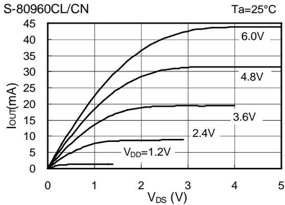
**6. Pch Transistor Output Current ( $I_{OUT}$ ) -  $V_{DS}$**
