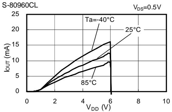
**8. Pch Transistor Output Current ( $I_{OUT}$ ) - Input Voltage ( $V_{DD}$ )**
