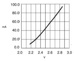
Forward Current vs Forward Voltage
