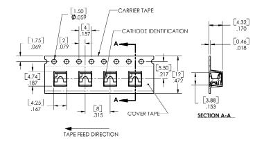
DIMENSIONS ARE IN INCHES AND [MILLIMETERS].
