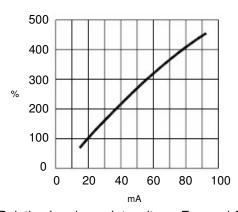
Relative Luminous Intensity vs Forward Current
