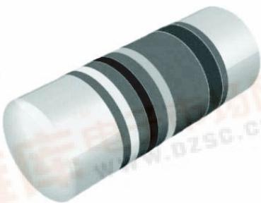
CMB 0207 speciality MELF resistors with advanced pulse load capability are the perfect choice for the protection of circuitry with signal and mains input lines from surge pulses. The resistors are also suitable for circuits exposed to high levels of electromagnetic interference or electro-static discharge. The applications are in all fields of automotive, telecommunication, industrial and medical equipment.
