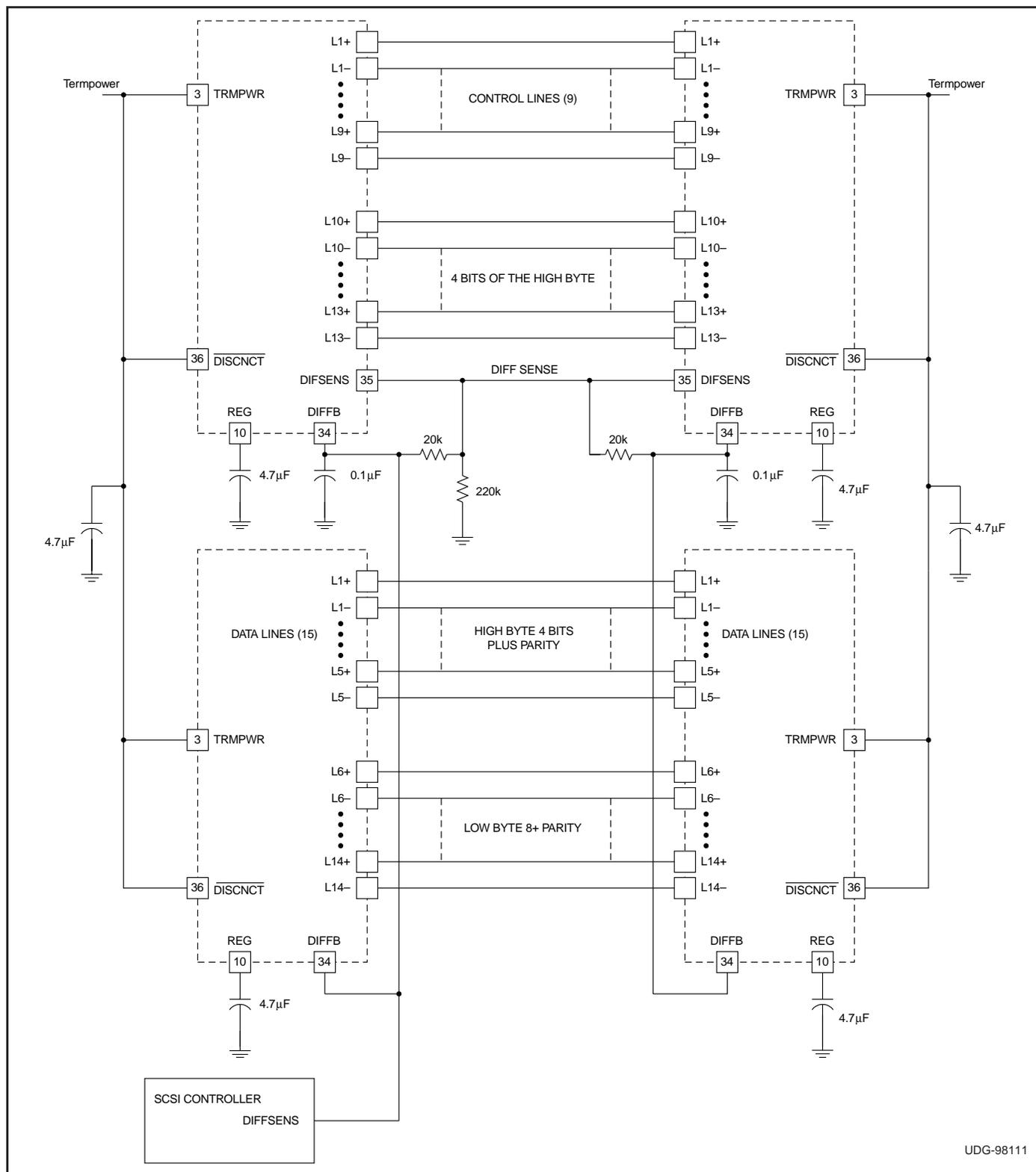
**Note:** A 220k resistor is added to ground to insure the transceivers will come up in single-ended mode when no terminator is enabled. The controller DIFFSENS ties to the DIFFFB pin on the terminators, only one RC network should be on a device.
