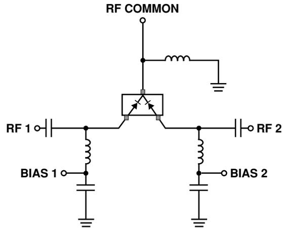
Figure 12. Simple SPDT Switch, Using Only Positive Current.
