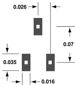
Figure 23. PCB Pad Layout, SOT-323. (dimensions in inches).
