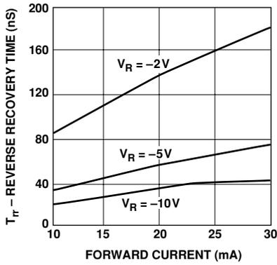
Figure 4. Typical Reverse Recovery Time vs. Reverse Voltage.
