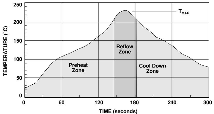
Figure 26. Surface Mount Assembly Profile.
