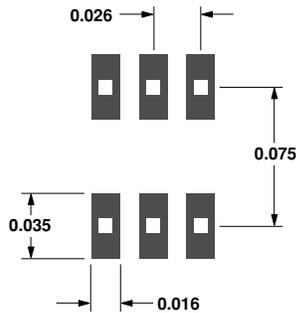
Figure 22. PCB Pad Layout, SOT-363. (dimensions in inches).
