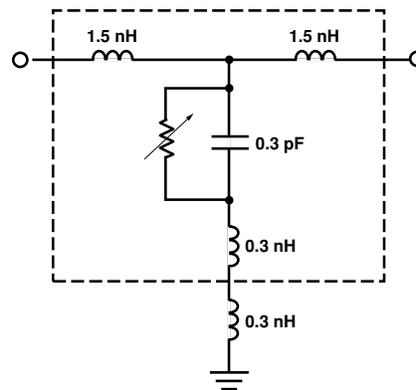
Figure 19. Equivalent Circuit.
