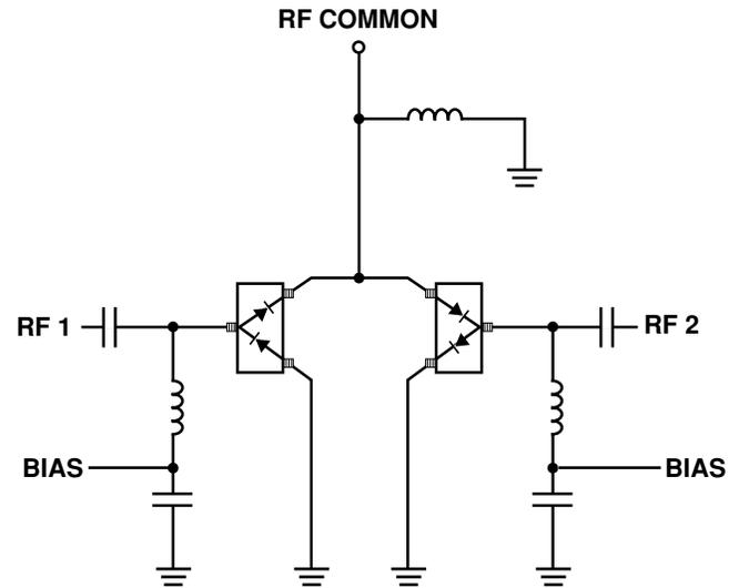
Figure 13. High Isolation SPDT Switch, Dual Bias.
