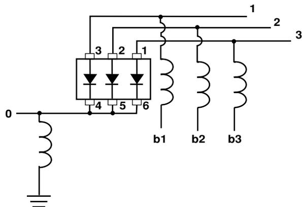
Figure 6. HSMP-389L used in a SP3T Switch.
