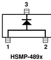
Figure 16. Internal Connections.
