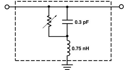
Figure 21. Equivalent Circuit.
