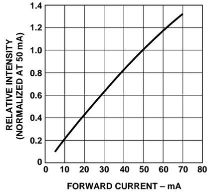
Figure 3. Relative Intensity Vs. Forward Current (AlInGaP).
