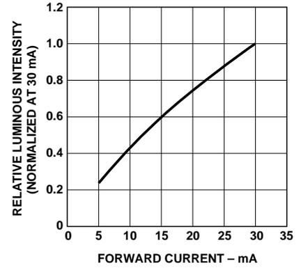
Figure 4. Relative Intensity Vs. Forward Current (InGaN).
