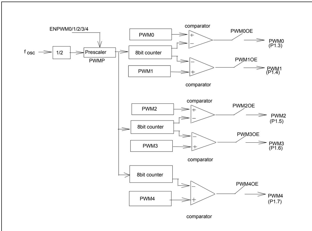
FIGURE 1 PWM DIAGRAM
