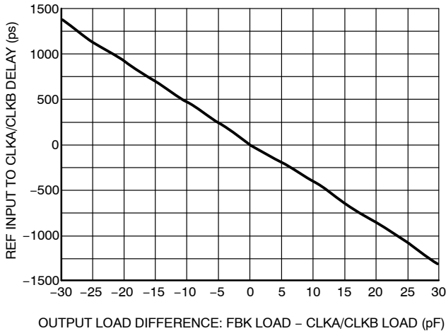
Figure 3. REF Input to CLKA/CLKB Delay vs. Difference in Loading between FBK Pin and CLKA/CLKB Pins
