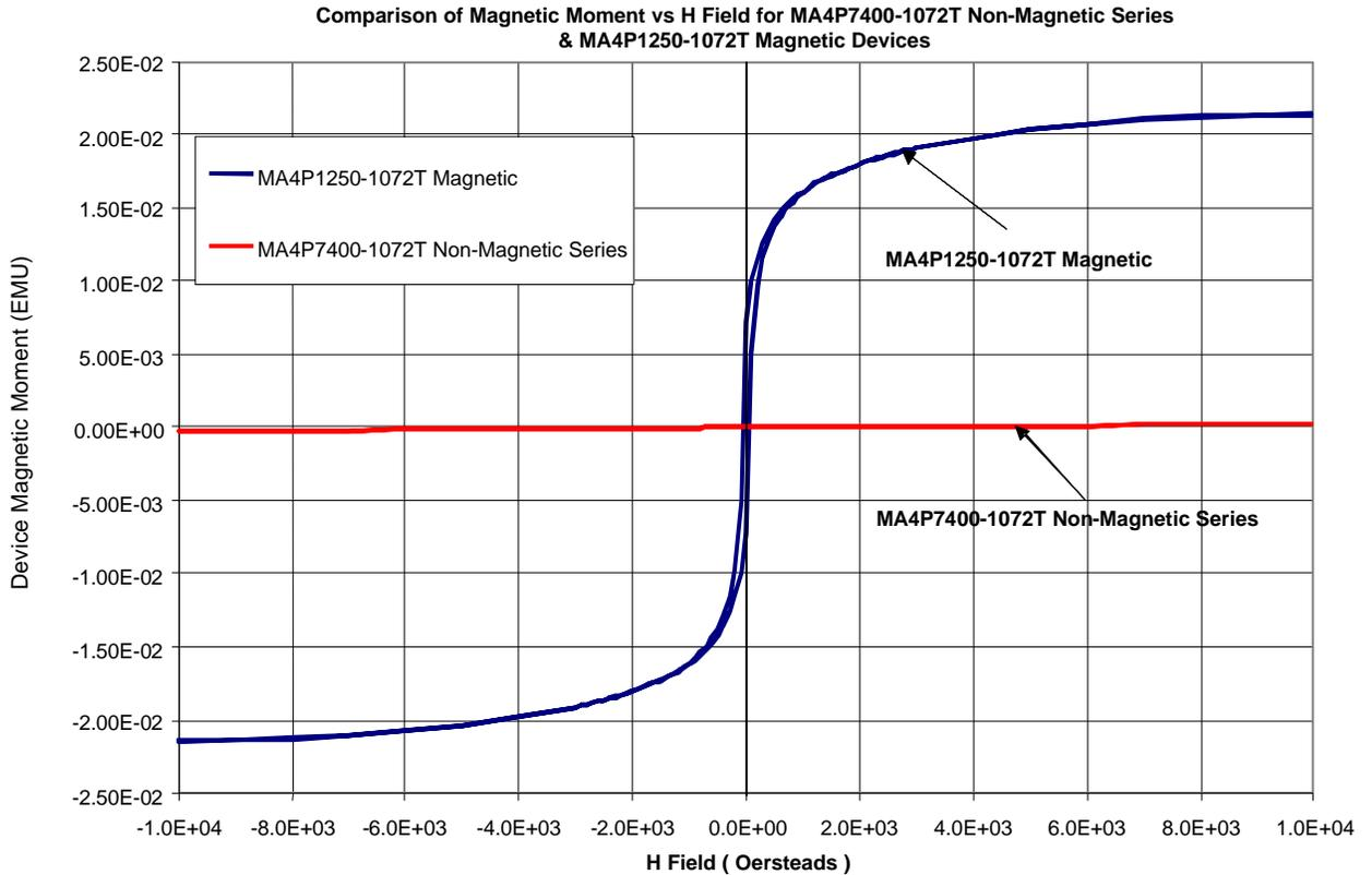
**Table 1 - Typical Magnetic Properties of Non-Magnetic MA4P7470F-1072T Device Vs. Conventional MA4P1250-1072T Magnetic Device**
