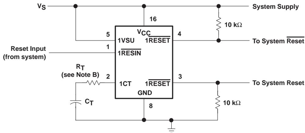
NOTE B: When  $V_{CC}$  and  $1VSU$  are connected to the same point, it is recommended that series resistance ( $R_T$ ) be added between the time-delay programming capacitor ( $C_T$ ) and the voltage-supervisor device terminal ( $1CT$ ). The suggested  $R_T$  value is given by:
