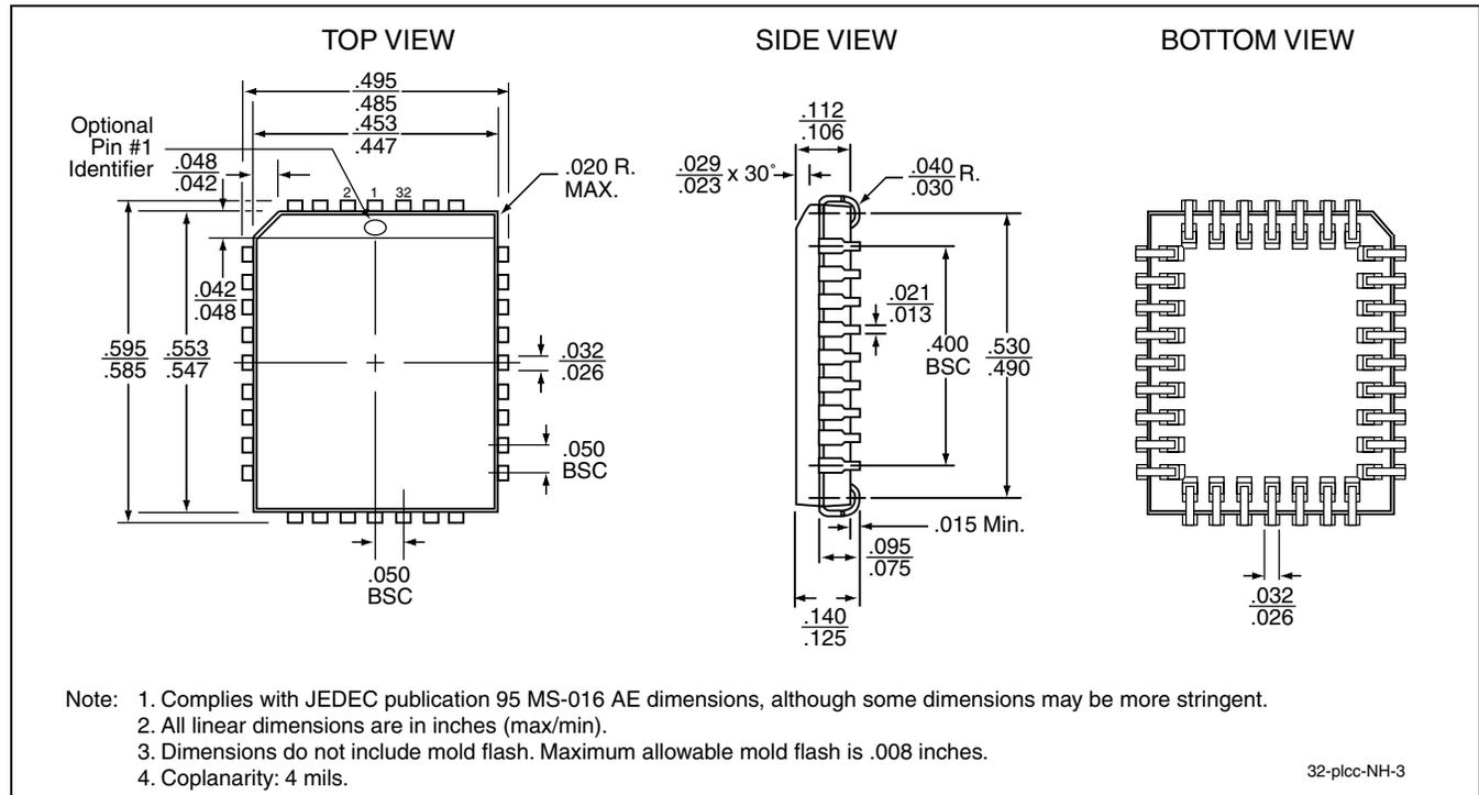
**32-LEAD PLASTIC LEAD CHIP CARRIER (PLCC)**
