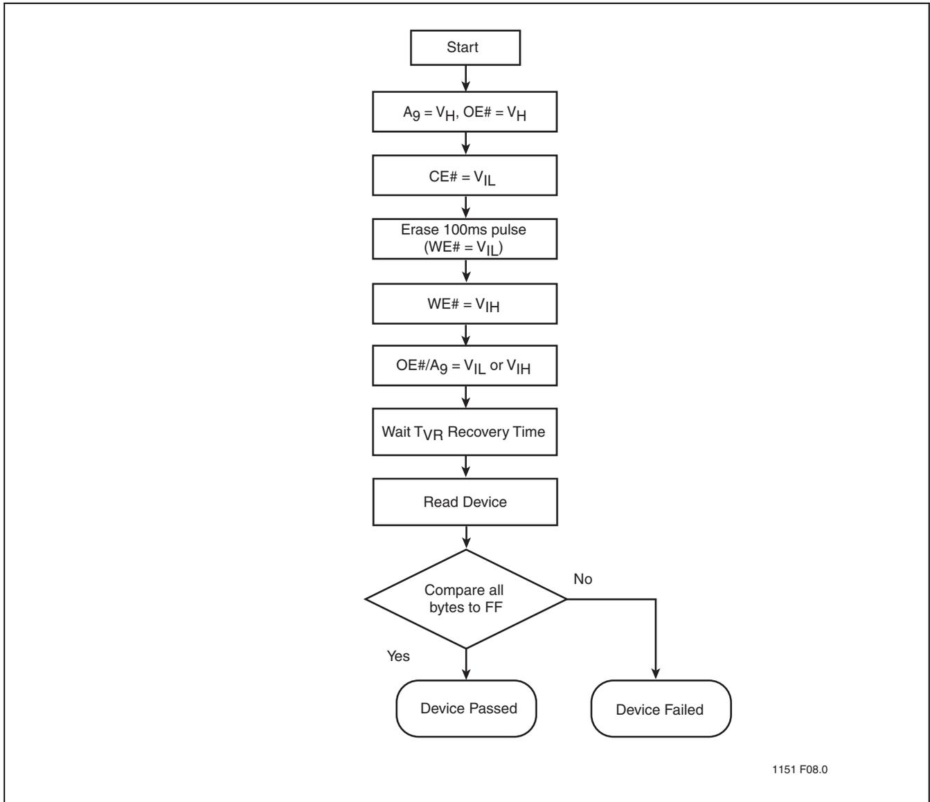
FIGURE 10: Chip-Erase Algorithm
