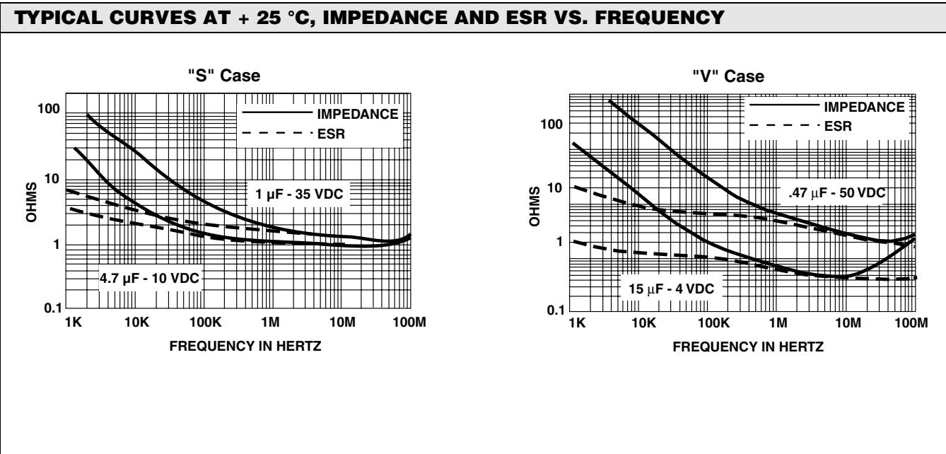
**TYPICAL CURVES AT + 25 °C, IMPEDANCE AND ESR VS. FREQUENCY**
