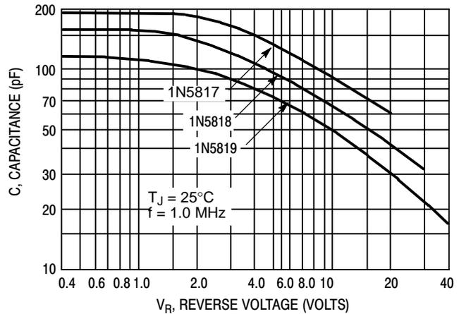
Figure 10. Typical Capacitance
