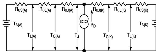
Use of the above model permits junction to lead thermal resistance for any mounting configuration to be found. For a given total lead length, lowest values occur when one side of the rectifier is brought as close as possible to the heatsink. Terms in the model signify:
