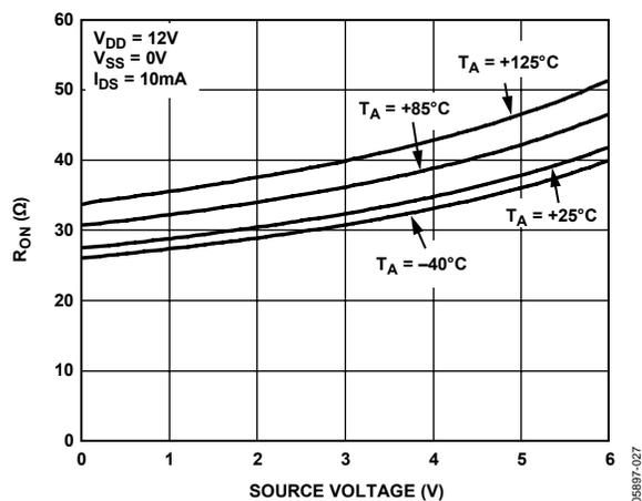
Figure 9.  $R_{ON}$  vs. Temperature,  $V_{DD} = 12\text{V}$
