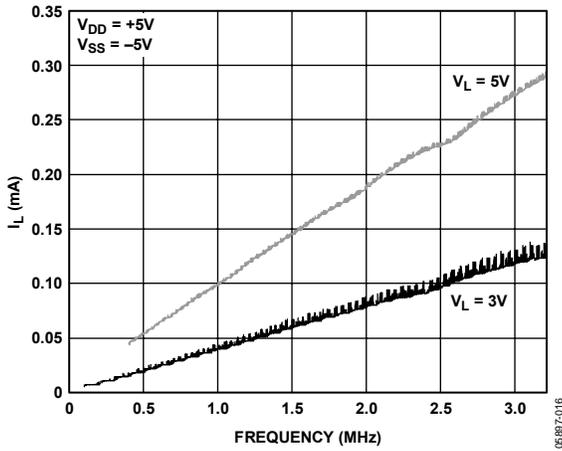
Figure 22. Digital Current ( $I_L$ ) vs. Frequency
