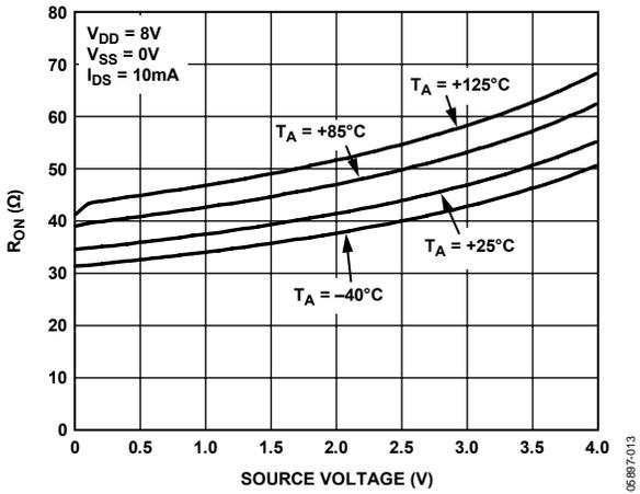
Figure 10.  $R_{ON}$  vs. Temperature,  $V_{DD} = 8V$
