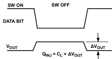
Figure 29. Charge Injection
