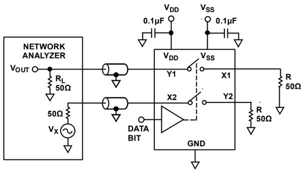
$$\text{CHANNEL-TO-CHANNEL CROSSTALK} = 20 \log \frac{V_{\text{OUT}}}{V_s}$$
