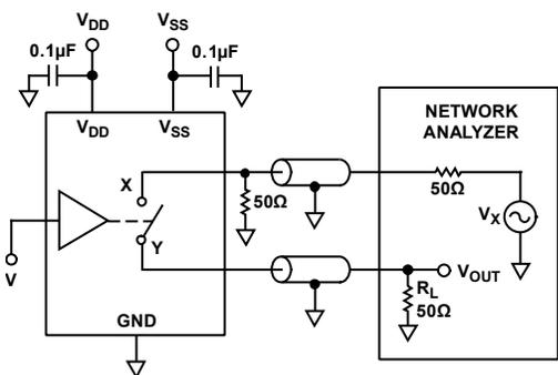
$$\text{OFF ISOLATION} = 20 \log \frac{V_{OUT}}{V_S}$$
