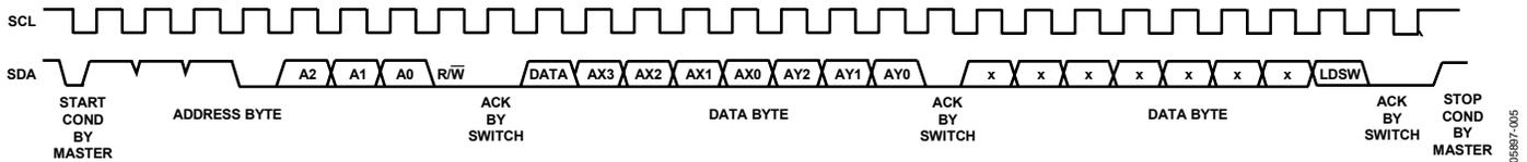
Figure 34. Write Operation
