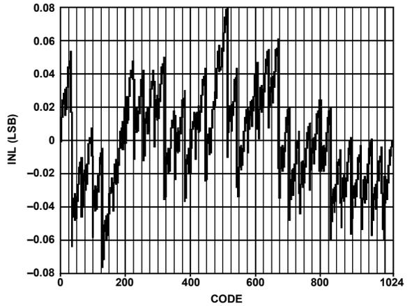
Figure 61. AD9705 Typical Uncalibrated INL
