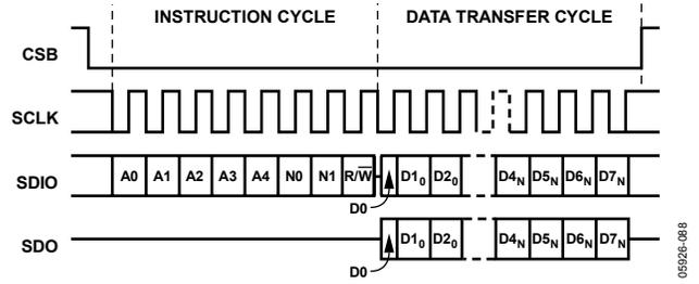
Figure 76. Serial Register Interface Timing, LSB First Read
