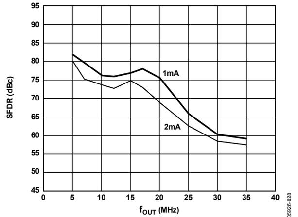
Figure 32. SFDR vs. f<sub>OUT</sub> and I<sub>OUTFS</sub> @ 80 MSPS
