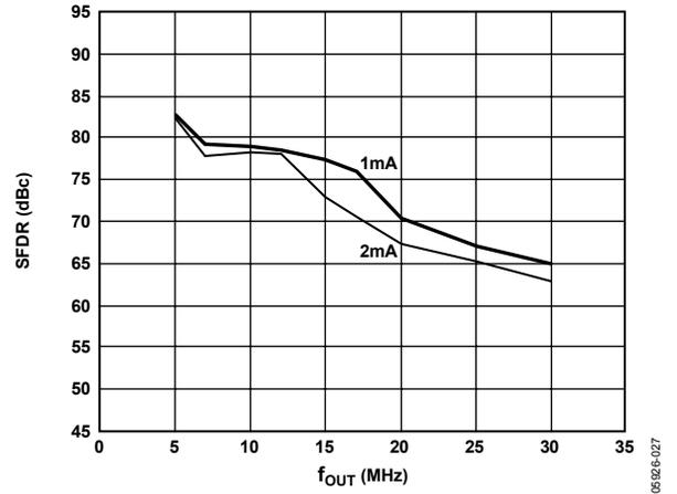
Figure 31. SFDR vs. f<sub>OUT</sub> and I<sub>OUTFS</sub> @ 65 MSPS
