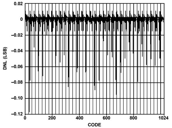
Figure 62. AD9705 Typical Uncalibrated DNL
