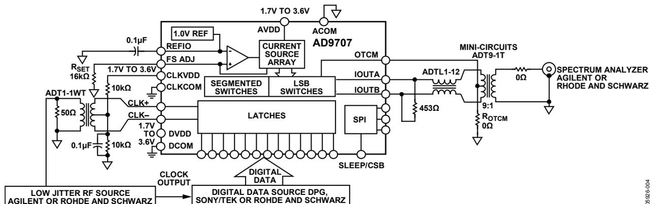
Figure 71. Basic AC Characterization Test Setup
