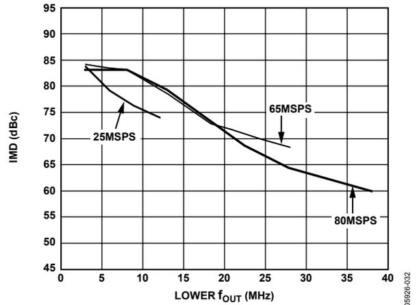
Figure 36. Dual-Tone IMD vs.  $f_{OUT}$  @  $I_{OUTFS} = 2 \text{ mA}$  and  $0 \text{ dBFS}$
