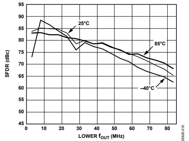
Figure 18. Dual-Tone IMD vs.  $f_{OUT}$  and Temperature @ 0 dBFS
