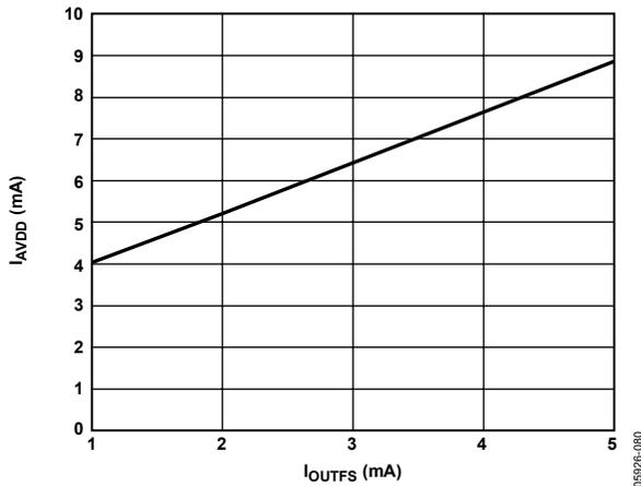
Figure 82.  $I_{AVDD}$  vs.  $I_{OUTFS}$  @  $AVDD = 3.3$  V
