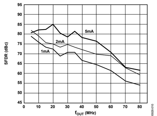
Figure 12. SFDR vs. f<sub>OUT</sub> and I<sub>OUTFS</sub> @ 175 MSPS
