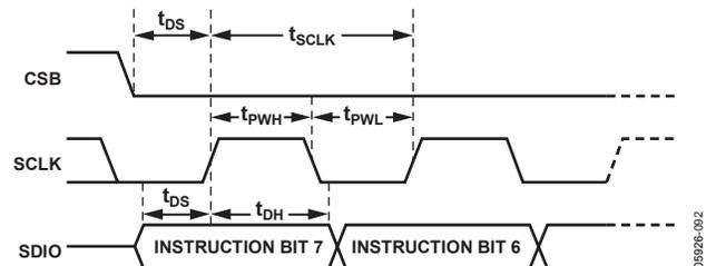
Figure 77. Timing Diagram for SPI Register Write
