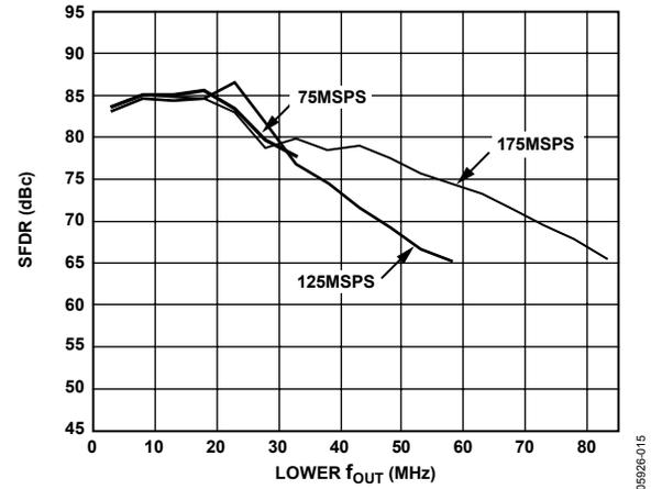
Figure 17. Dual-Tone IMD vs.  $f_{OUT}$  @ 0 dBFS
