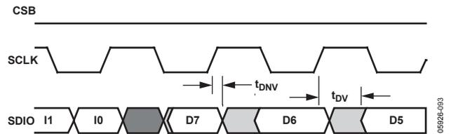
Figure 78. Timing Diagram for SPI Register Read
