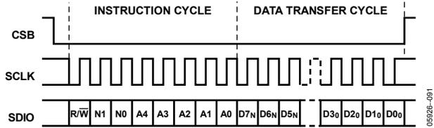
Figure 73. Serial Register Interface Timing, MSB First Write
