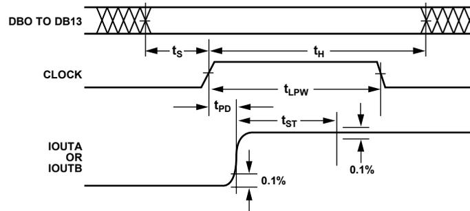
Figure 2. Timing Diagram
