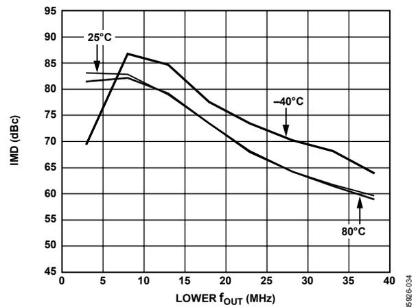
Figure 38. Dual-Tone IMD vs.  $f_{OUT}$  and Temperature @  $80 \text{ MSPS}$ ,  $I_{OUTFS} = 2 \text{ mA}$  and  $0 \text{ dBFS}$
