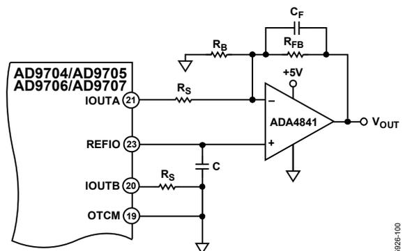
Figure 91. Single-Supply Single-Ended Buffer
