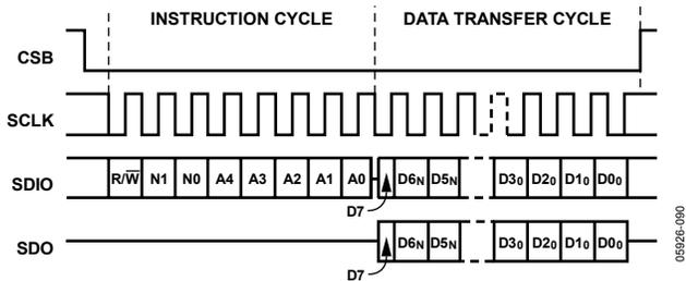
Figure 74. Serial Register Interface Timing, MSB First Read
