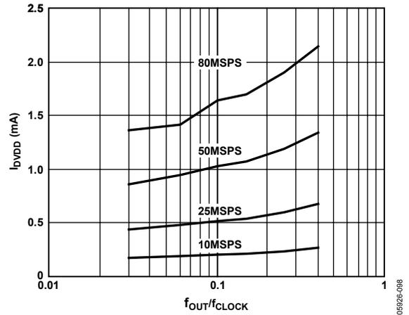
Figure 85.  $I_{DVDD}$  vs.  $f_{OUT}/f_{CLOCK}$  Ratio @  $DVDD = 1.8$  V
