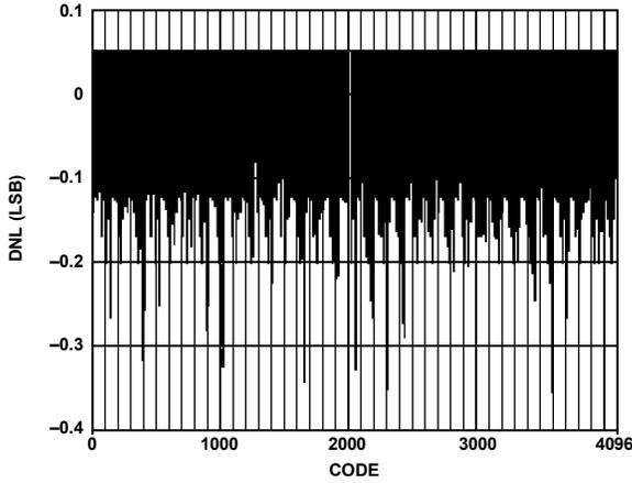
Figure 64. AD9706 Typical Uncalibrated DNL
