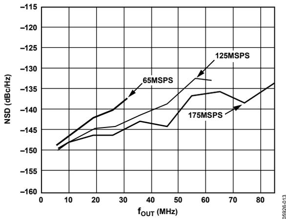
Figure 15. NSD vs.  $f_{OUT}$  and  $f_{CLOCK}$  @ 0 dBFS
