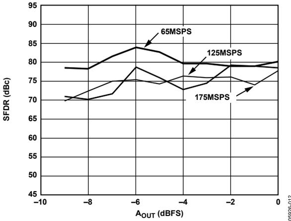
Figure 14. Single-Tone SFDR vs.  $A_{OUT}$  @  $f_{OUT} = f_{CLOCK}/5$
