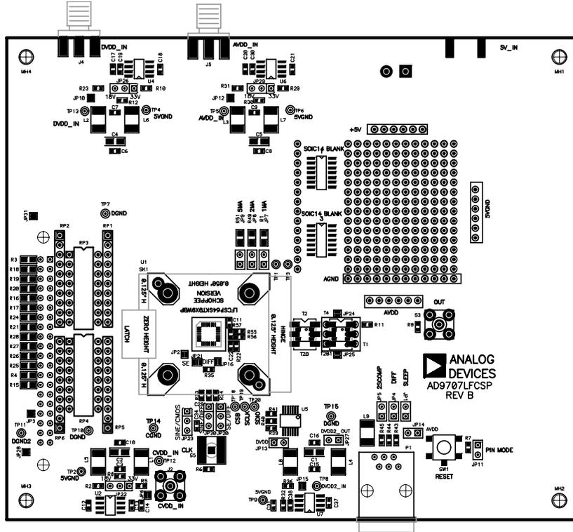
Figure 98. Assembly—Primary Side
