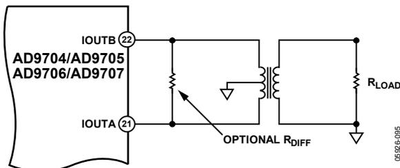
Figure 90. Differential Output Using a Transformer
