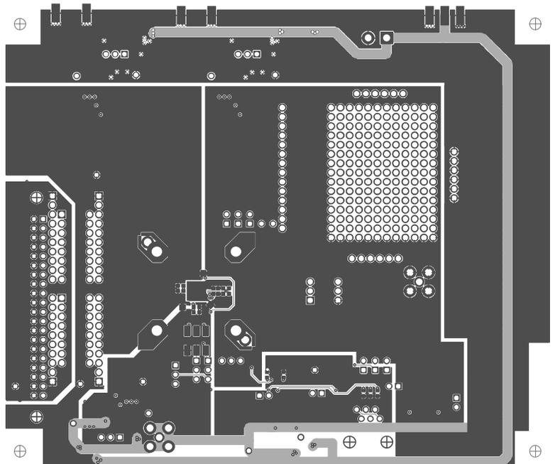
Figure 101. Layer 4—Secondary Side
