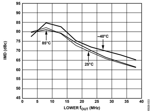
Figure 37. Dual-Tone IMD vs.  $f_{OUT}$  and Temperature @  $80 \text{ MSPS}$ ,  $I_{OUTFS} = 1 \text{ mA}$  and  $0 \text{ dBFS}$
