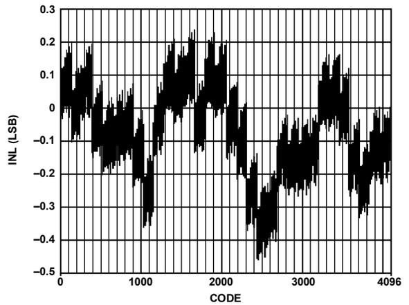
Figure 63. AD9706 Typical Uncalibrated INL
