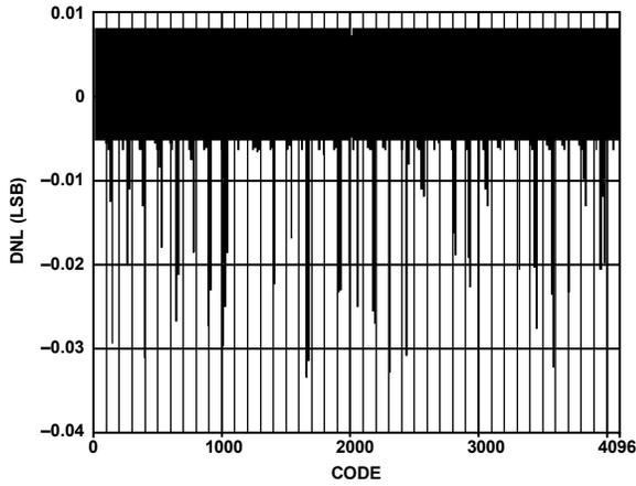
Figure 51. AD9706 Typical Uncalibrated DNL
