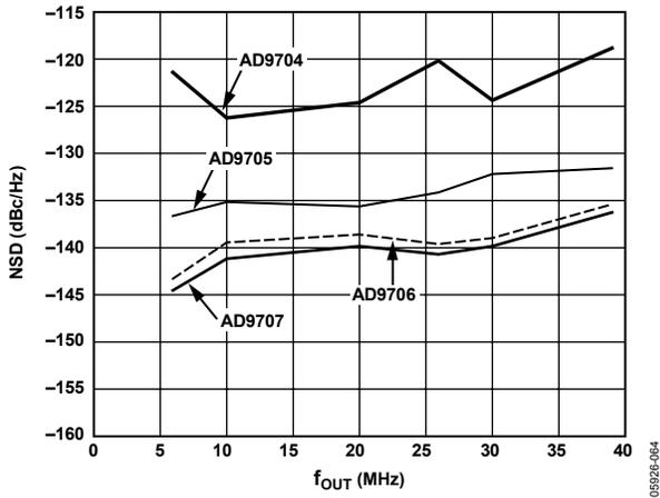
Figure 58. AD9704, AD9705, AD9706 NSD vs.  $f_{OUT}$  @ 0 dBFS
