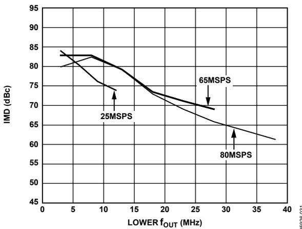
Figure 35. Dual-Tone IMD vs.  $f_{OUT}$  @  $I_{OUTFS} = 1 \text{ mA}$  and  $0 \text{ dBFS}$
