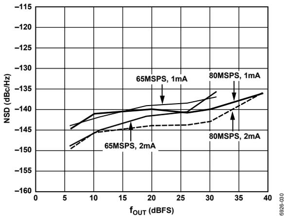
Figure 34. NSD vs.  $f_{OUT}$ ,  $f_{CLOCK}$ , and  $I_{OUTFS}$  @  $0 \text{ dBFS}$
