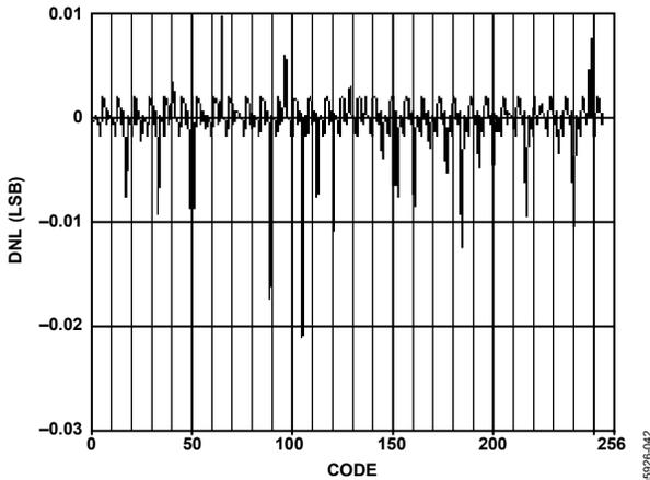
Figure 47. AD9704 Typical Uncalibrated DNL
