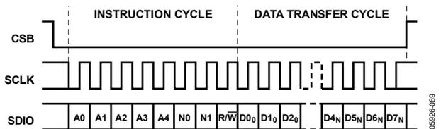
Figure 75. Serial Register Interface Timing, LSB First Write
