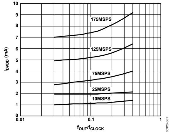
Figure 84.  $I_{DVDD}$  vs.  $f_{OUT}/f_{CLOCK}$  Ratio @  $DVDD = 3.3$  V
