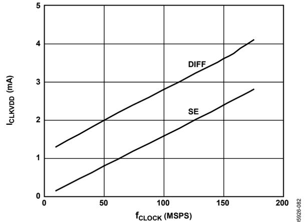
Figure 86.  $I_{CLKVDD}$  vs.  $f_{CLOCK}$  @  $CLKVDD = 3.3$  V
