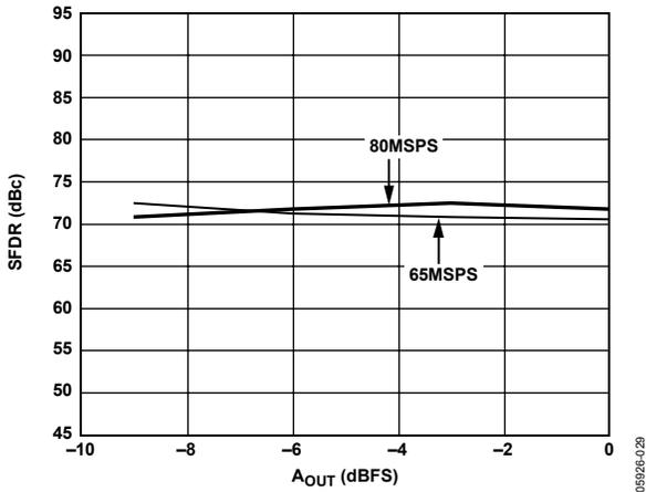
Figure 33. Single-Tone SFDR vs.  $A_{OUT}$  @  $f_{OUT} = f_{CLOCK}/5$
