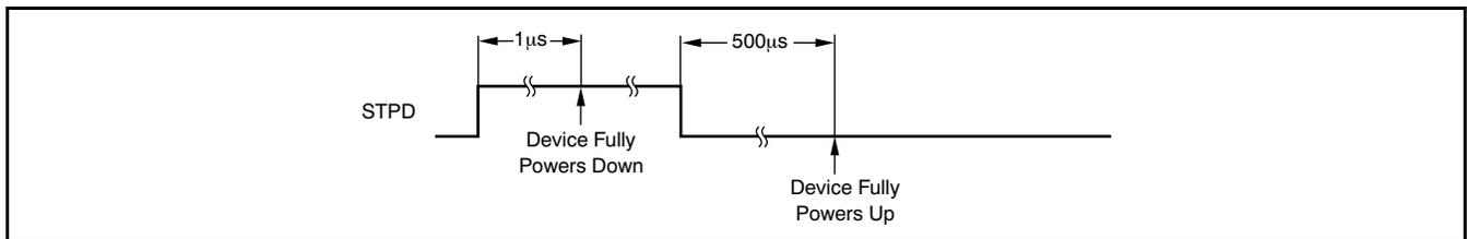
NOTE: The shown power-up time is based on 1 $\mu\text{F}$  bypass capacitors on the reference pins. See the [Theory of Operation](#) section for details.
