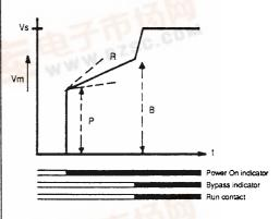
P should be set at minimum initially (fully anticlockwise). After the supply is turned on, P can be turned slowly clockwise until the motor commences rotating with the maximum shaft loading expected.
