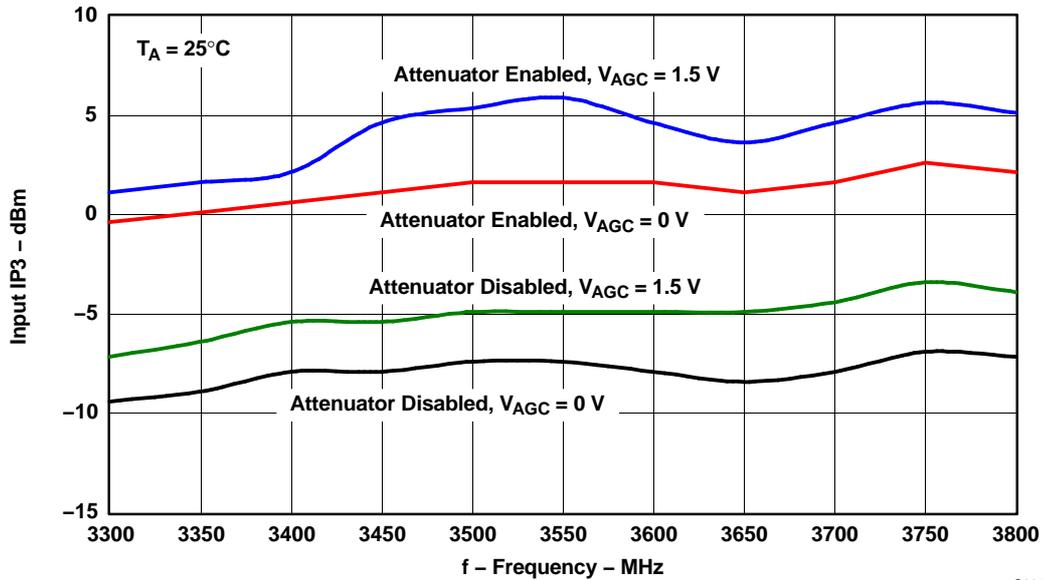
Figure 6. Input IP3 vs Frequency, (T<sub>A</sub> = 25°C)
