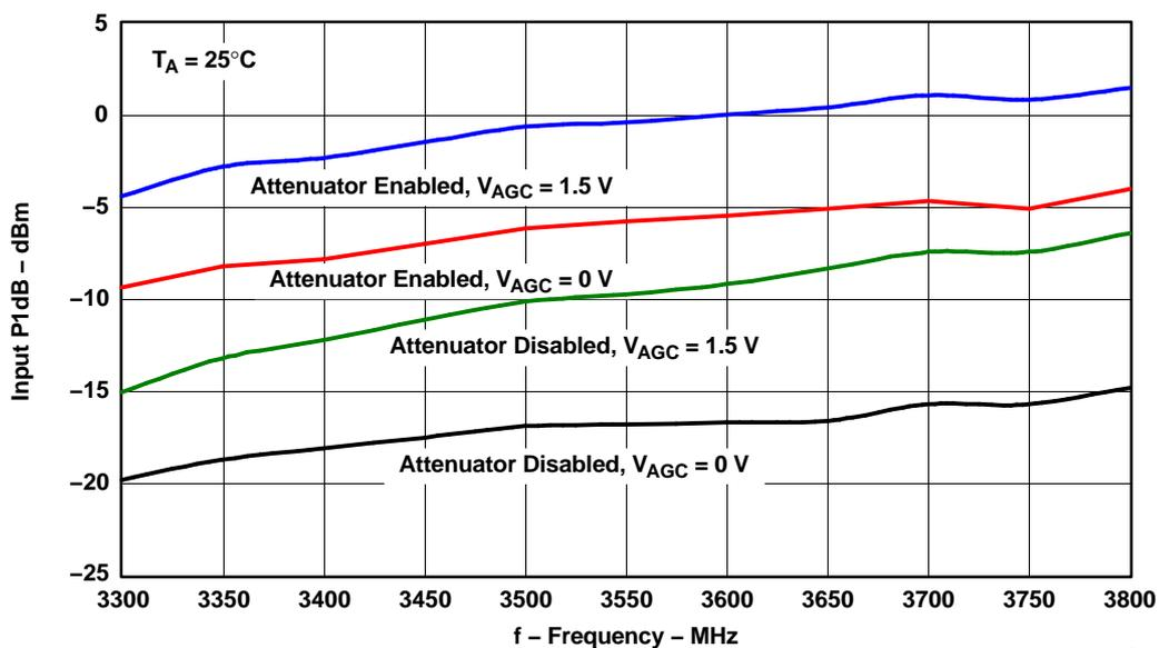
Figure 5. Input P1dB vs Frequency, (T<sub>A</sub> = 25°C)
