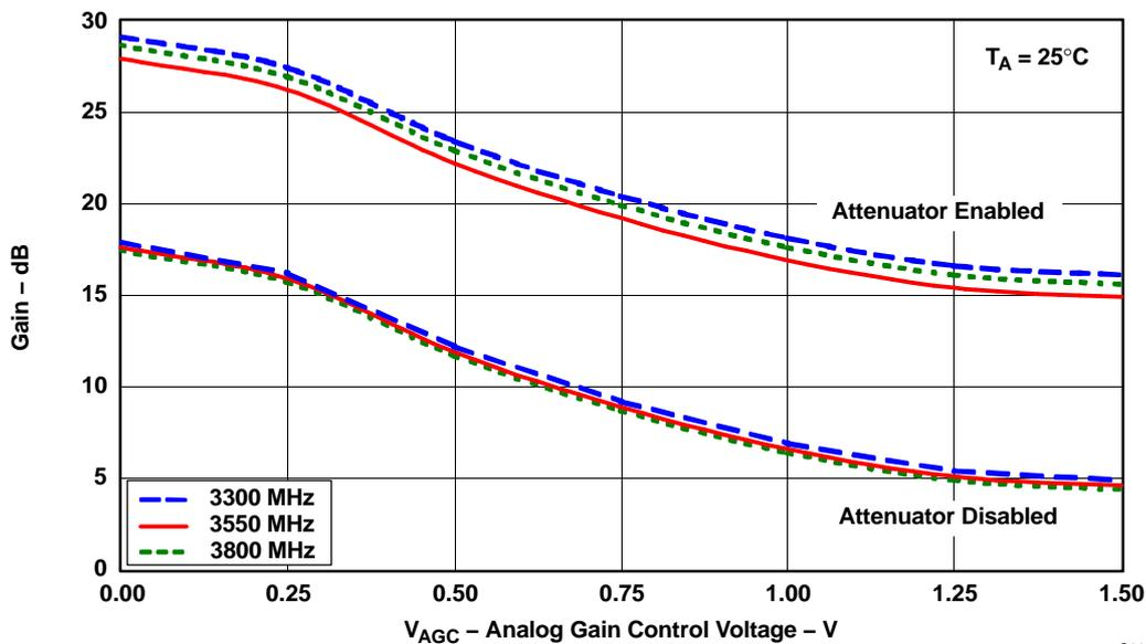
Figure 4. Gain vs VAGC for Different Frequencies, (T<sub>A</sub> = 25°C)
