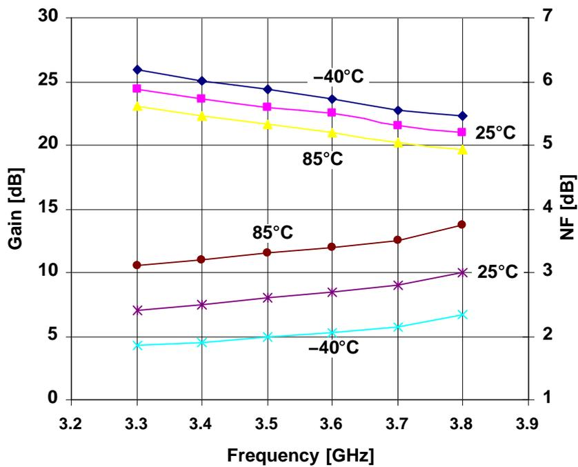
Figure 7. LNA Noise Figure vs Frequency With V<sub>AGC</sub> = 0 V
