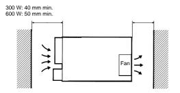
Take care to minimize dirt, dust, and other air-borne debris which could interfere with the passage of cooling air.
