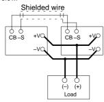
In master/slave operation, the Power Supply with the lower voltage adjustment set value (controlled by V. ADJ) is the master unit, and the Power Supply with the higher voltage adjustment set value is the slave unit.
