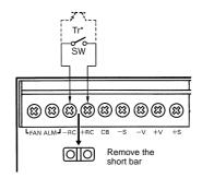
\*Use a transistor with  $V_{CE} > 20$  V and  $I_C > 5$  mA.
