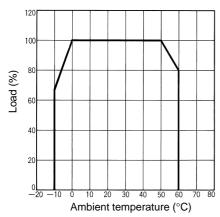
Note: The derating curve differs depending on the mounting direction of the Power Supply. The curve above was obtained with the Power Supply mounted in the standard position.
