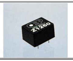
Provides isolation between modems or similar devices and telephone lines. This transformer is designed for use in voice or data transmission circuits where the line d.c. is diverted from the windings by a choke or solid state device. The use of this transformer should enable the equiptment it is used with to cpmly with the relevent requirments of BS6305. This is a lower profile version of the OEP 1200 transformer.
