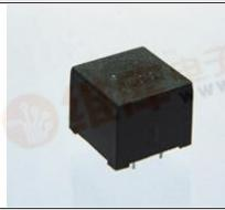
Provides isolation between modems or similar devices and telephone lines. This transformer is designed for use in voice or data transmission circuits where the line d.c. is diverted from the windings by a choke or solid state device. The use of this transformer should enable the equipment it is used with to comply with the relevant requirements of BS6305.
