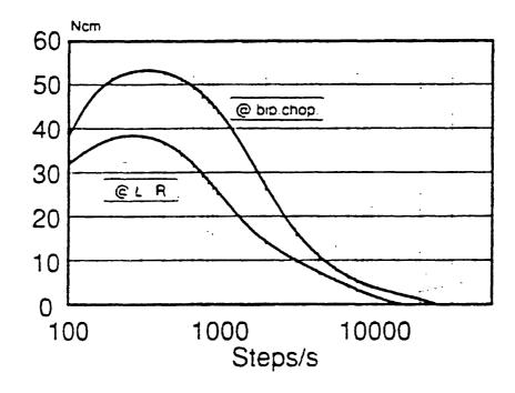
DRIVE: BIPOLAR CHOPPER 35V - 1.4 A/ph DRIVE: UNIPOLAR L/R 35V - Rs =29 OHM
