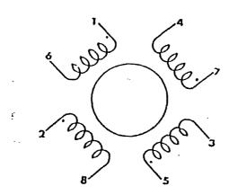
REVISED CONNECTION DETAILS FOR STEPPER MOTOR TYPE Y163/4 AS FROM PRODUCTION BATCH RECEIVED 22.04.97
