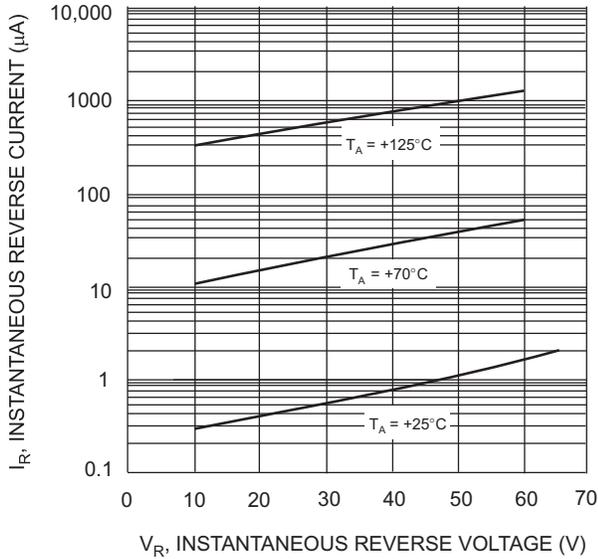
Fig. 7 Typical Reverse Characteristics, B150/B thru B160/B
