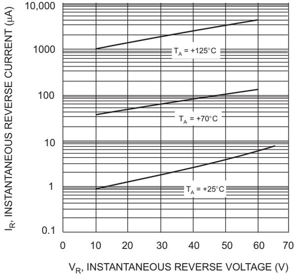
Fig. 7 Typical Reverse Characteristics, B350A thru B360A
