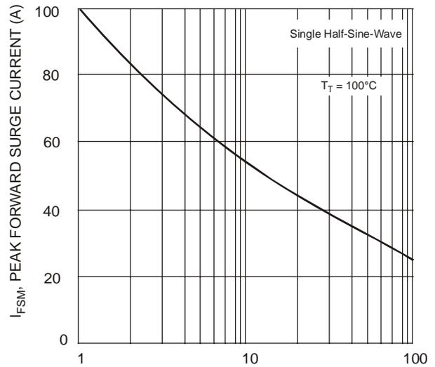
Fig. 4 Max Non-Repetitive Peak Forward Surge Current
