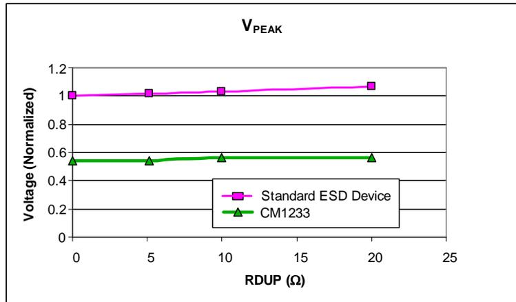
Figure 4. V<sub>Peak</sub> (8KV IEC-61000 4-2 ESD Contact Strike) and V<sub>Clamp</sub> vs. Loading (RDUP)\*
