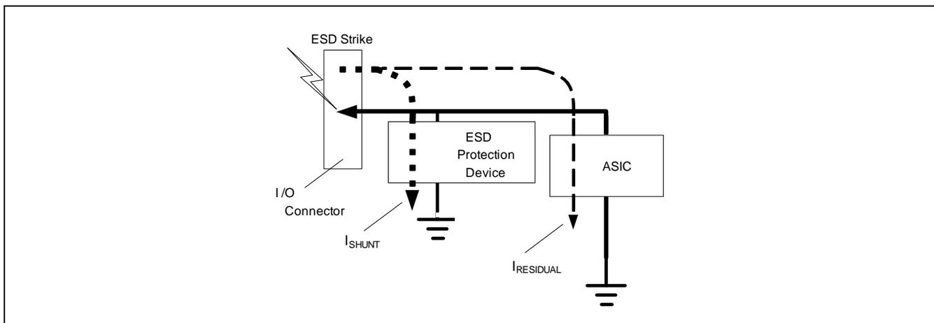
Figure 1. Standard ESD Protection Device Block Diagram
