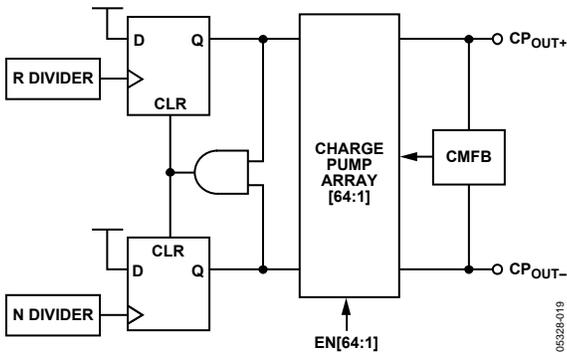
Figure 23. PFD and Differential Charge Pump Simplified Schematic
