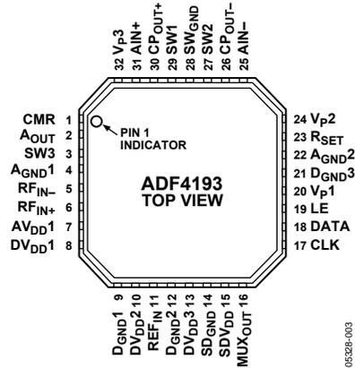
Figure 3. Pin Configuration
