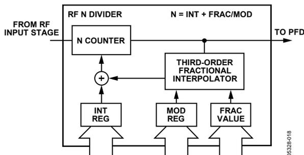
Figure 22. Fractional-N Divider
