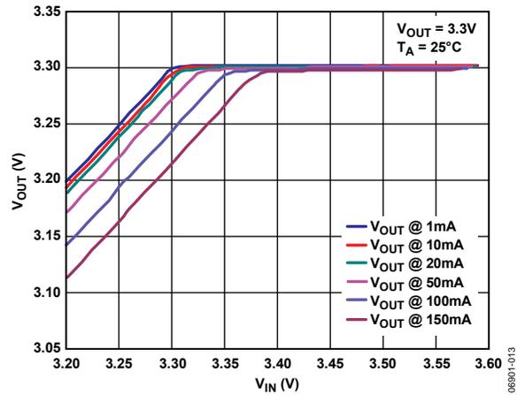
Figure 15. Output Voltage vs. Input Voltage (In Dropout), WLCS
