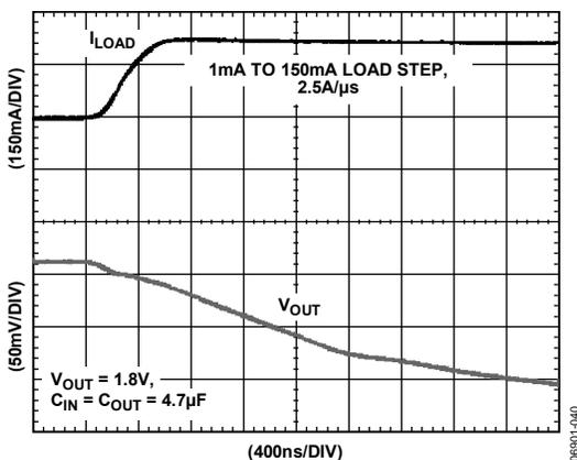
Figure 29. Output Transient Response,  $C_{OUT} = 4.7\ \mu\text{F}$
