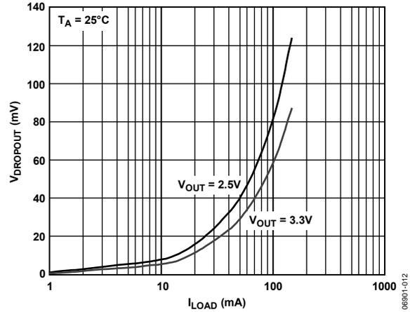
Figure 14. Dropout Voltage vs. Load Current, WLCS
