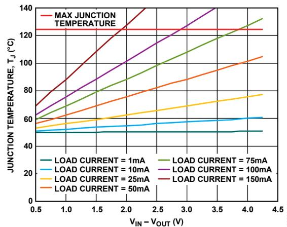
Figure 45. WLCSP, 0 mm<sup>2</sup> of PCB Copper,  $T_A = 50^\circ\text{C}$
