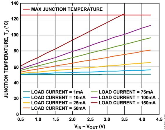
Figure 38. TSOT, 100 mm<sup>2</sup> of PCB Copper, T<sub>A</sub> = 50°C
