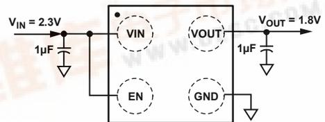
Figure 2. ADP121 WLCSP with Fixed Output Voltage, 1.8 V
