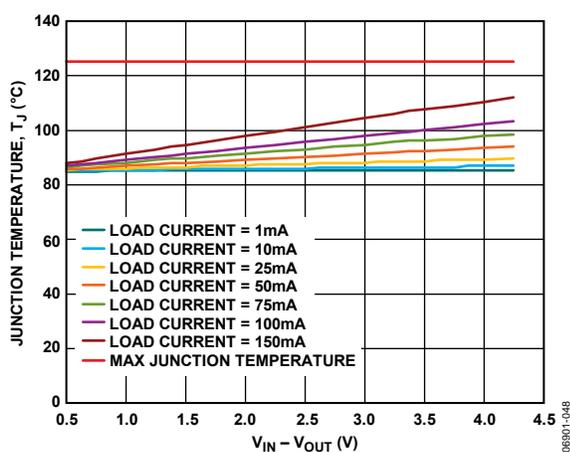
Figure 46. TSOT, 100 mm<sup>2</sup> of PCB Copper, T<sub>A</sub> = 85°C
