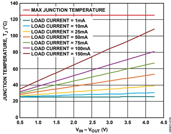
Figure 34. TSOT, 500 mm<sup>2</sup> of PCB Copper, T<sub>A</sub> = 25°C
