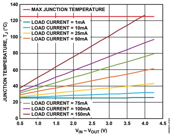
Figure 36. TSOT, 0 mm<sup>2</sup> of PCB Copper, T<sub>A</sub> = 25°C
