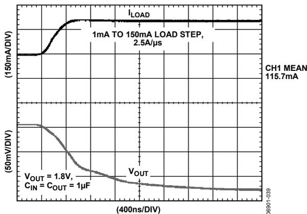
Figure 28. Output Transient Response,  $C_{OUT} = 1\ \mu\text{F}$
