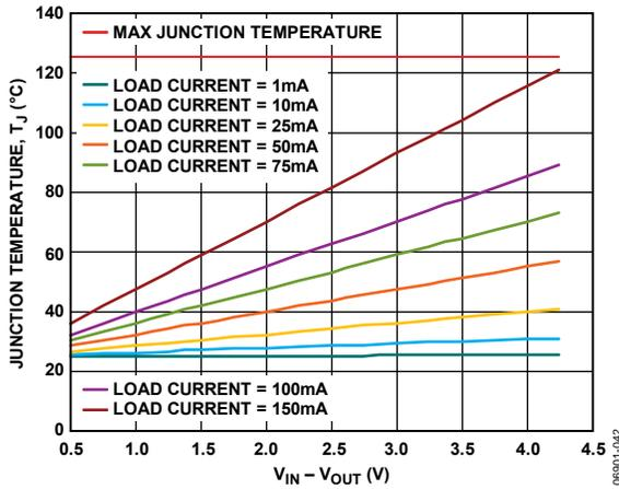
Figure 40. WLCSP, 500 mm<sup>2</sup> of PCB Copper,  $T_A = 25^\circ\text{C}$
