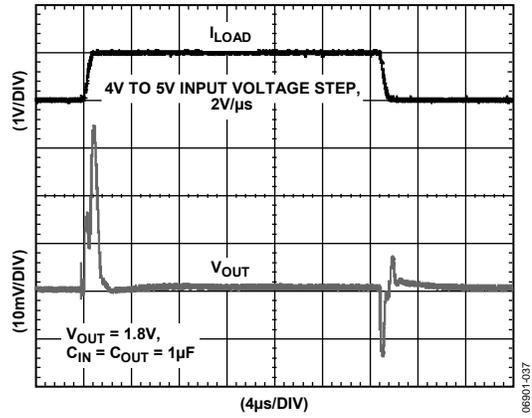
Figure 25. Line Transient Response, Load Current = 150 mA
