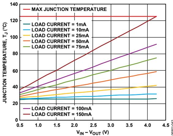
Figure 41. WLCSP, 100 mm<sup>2</sup> of PCB Copper,  $T_A = 25^\circ\text{C}$
