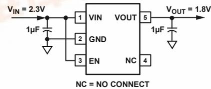
Figure 1. ADP121 TSOT with Fixed Output Voltage, 1.8 V
