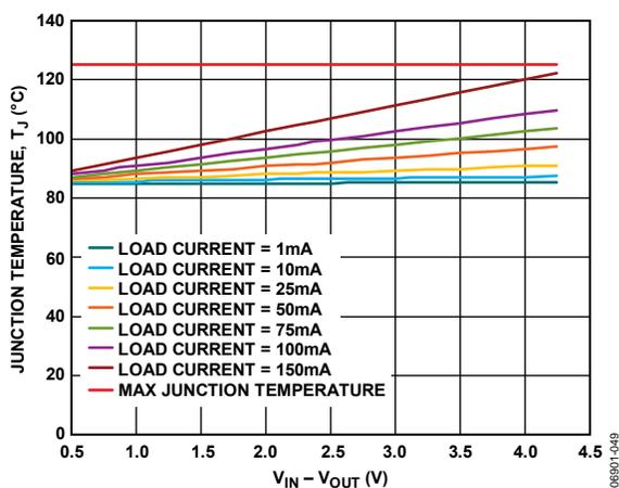
Figure 47. WLCSP, 100 mm<sup>2</sup> of PCB Copper, T<sub>A</sub> = 85°C
