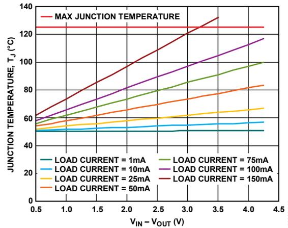
Figure 44. WLCSP, 100 mm<sup>2</sup> of PCB Copper,  $T_A = 50^\circ\text{C}$
