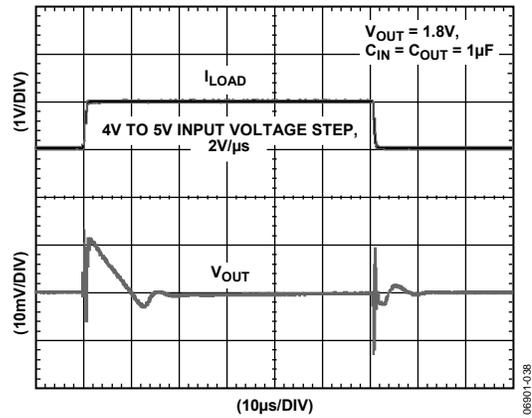
Figure 26. Line Transient Response, Load Current = 1 mA
