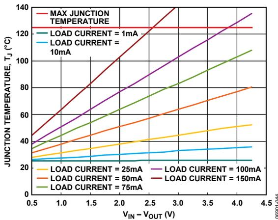
Figure 42. WLCSP, 0 mm<sup>2</sup> of PCB Copper,  $T_A = 25^\circ\text{C}$
