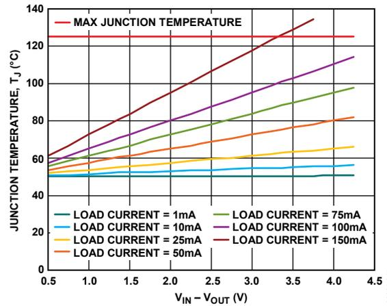
Figure 43. WLCSP, 500 mm<sup>2</sup> of PCB Copper,  $T_A = 50^\circ\text{C}$
