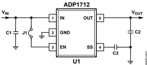
Figure 3. ADP1712 Fixed Output with Soft Start
