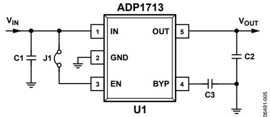
Figure 5. ADP1713 Fixed Output with Bypass
