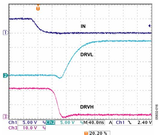
Figure 6. DRVH Fall and DRVL Rise Times
