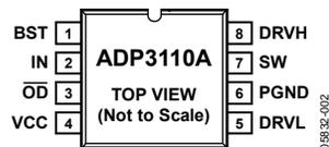
Figure 2. Pin Configuration
