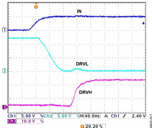
Figure 5. DRVH Rise and DRVL Fall Times
