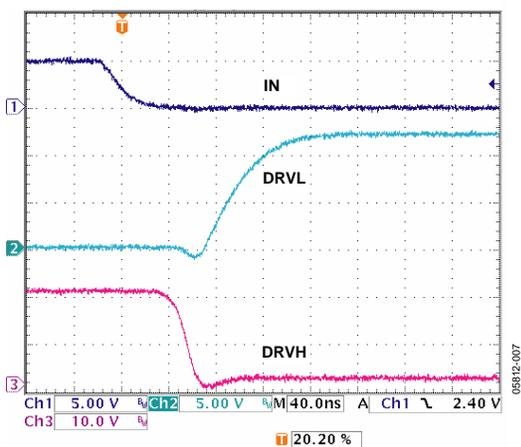
Figure 7. DRVH Fall and DRVL Rise Times
