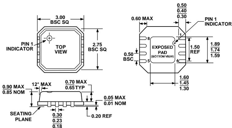
Figure 18. 8-Lead Lead Frame Chip Scale Package [LFCSP\_VD]
