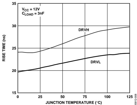
Figure 8. DRVH and DRVL Rise Times vs. Temperature
