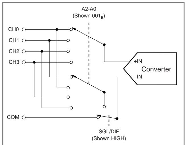
FIGURE 2. Simplified Diagram of the Analog Input.
