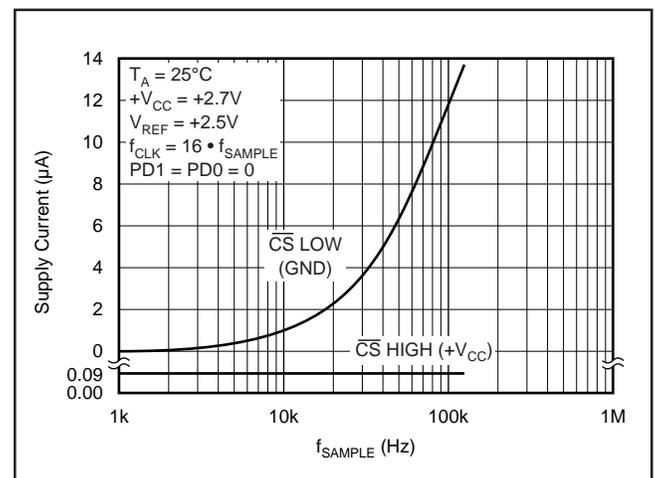
FIGURE 9. Supply Current vs State of  $\overline{\text{CS}}$ .
