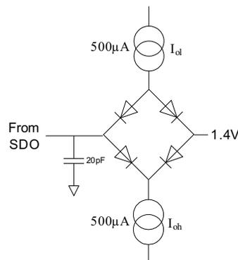
**Figure 1. Load Circuit for Digital Interface Timing**
