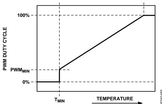
Figure 54. PWM<sub>MIN</sub> Determines Minimum PWM Duty Cycle
