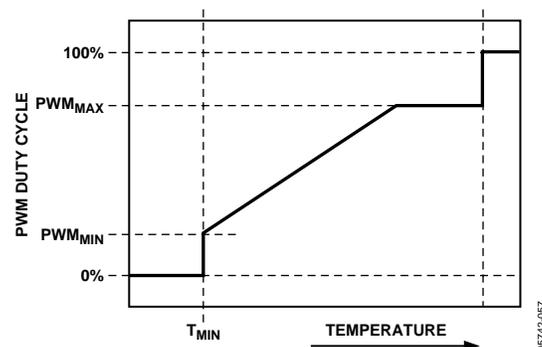
Figure 56. PWM<sub>MAX</sub> Determines Maximum PWM Duty Cycle Below the THERM Temperature Limit
