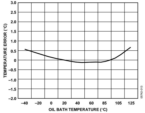
Figure 12. Remote Temperature Error vs. ADT7476A Temperature
