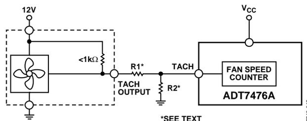
Figure 44. Fan with Strong TACH Pull-Up to > V<sub>CC</sub> or Totem-Pole Output, Attenuated with R<sub>1</sub>/R<sub>2</sub>
