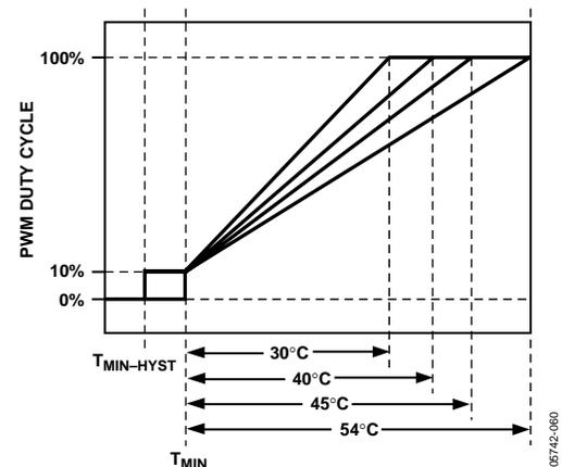
Figure 59. Increasing  $T_{RANGE}$  Changes the AFC slope
