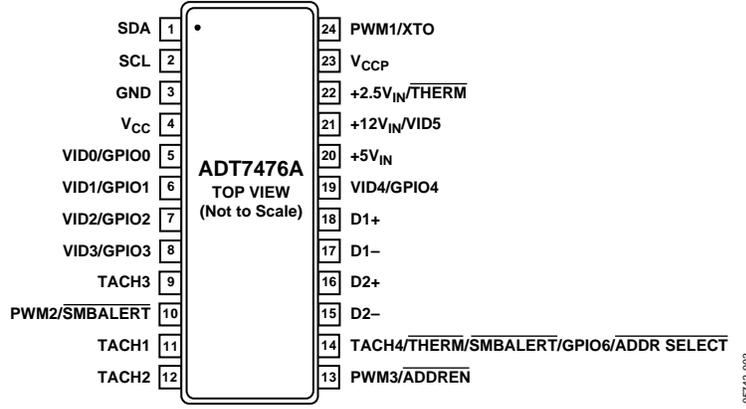
Figure 3. Pin Configuration
