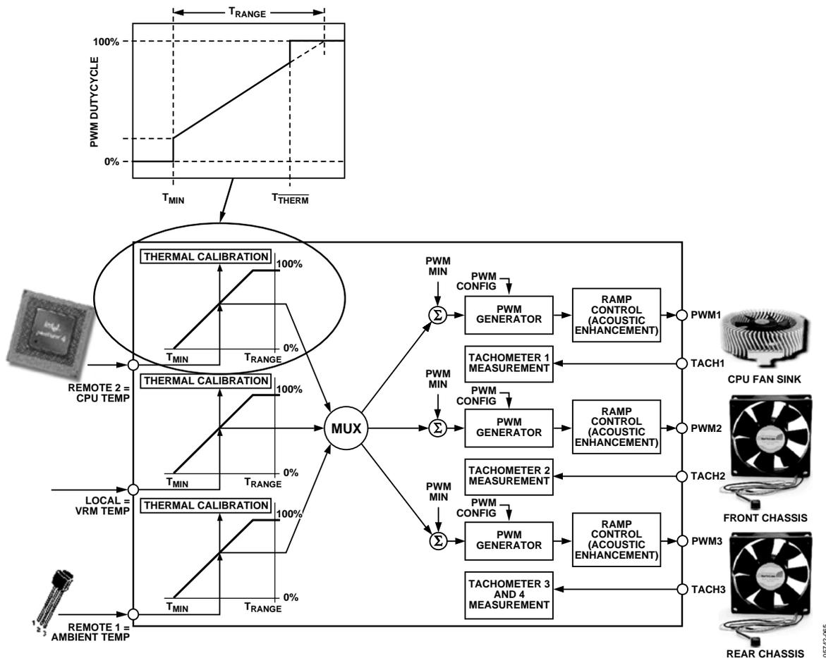
Figure 64. How  $T_{THERM}$  Relates to Automatic Fan Control
