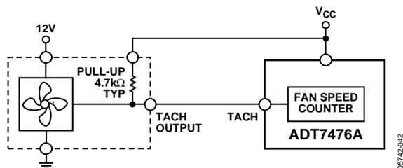
Figure 41. Fan with TACH Pull-Up to V<sub>CC</sub>
