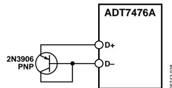
Figure 27. Measuring Temperature Using a PNP Transistor
