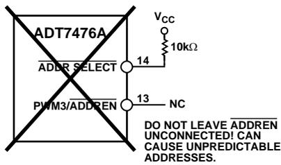
CARE SHOULD BE TAKEN TO ENSURE THAT PIN 13 (PWM3/ADDREN) IS EITHER TIED HIGH OR LOW. LEAVING PIN 13 FLOATING COULD CAUSE THE ADT7476A TO POWER UP WITH AN UNEXPECTED ADDRESS.
