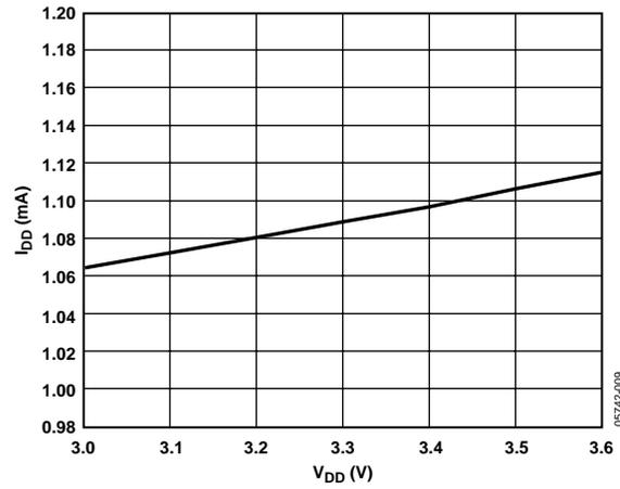
Figure 8. Normal I<sub>DD</sub> vs. Power Supply
