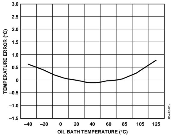
Figure 11. Internal Temperature Error vs. ADT7476A Temperature
