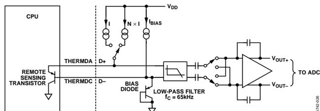
Figure 25. Signal Conditioning for Remote Diode Temperature Sensors
