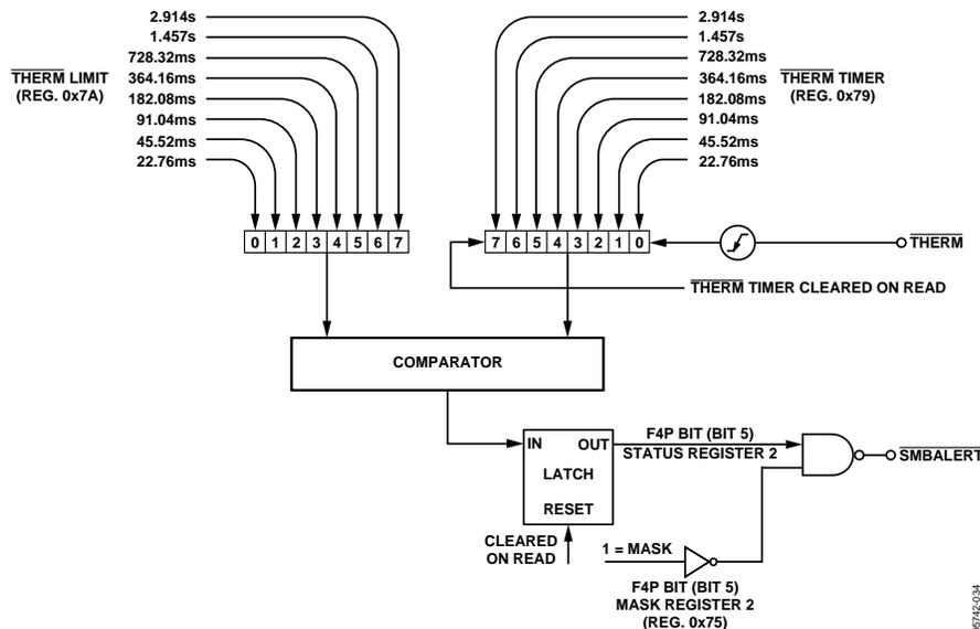
Figure 33. Functional Block Diagram of  $\overline{THERM}$  Monitoring Circuitry
