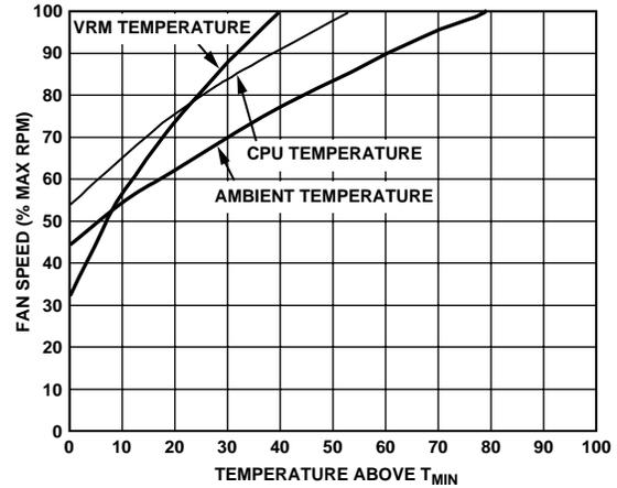
Figure 62.  $T_{RANGE}$  and % Fan Speed Slopes with  $PWM_{MIN} = 20\%$
