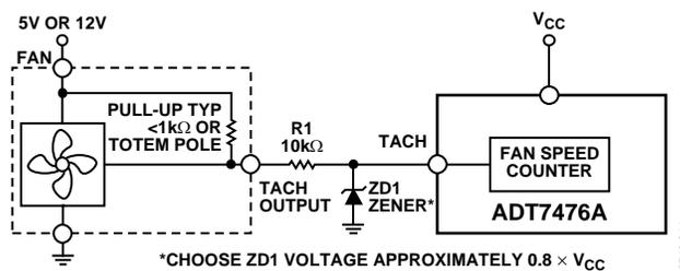
Figure 43. Fan with Strong TACH Pull-Up to > V<sub>CC</sub> or Totem-Pole Output, Clamped with Zener Diode and Resistor
