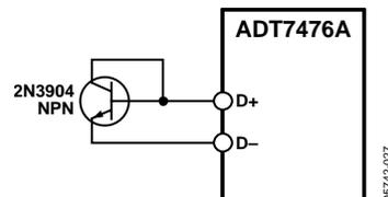
Figure 26. Measuring Temperature Using an NPN Transistor
