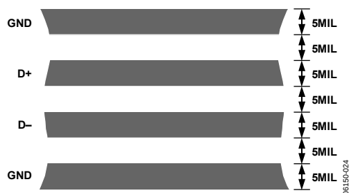
Figure 24. Typical Arrangement of Signal Tracks
