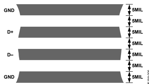
Figure 18. Arrangements of Signal Tracks
