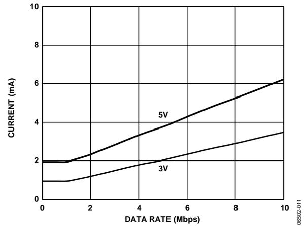
Figure 11. Typical ADuM1410 V<sub>DD1</sub> Supply Current vs. Data Rate for 5 V and 3 V Operation
