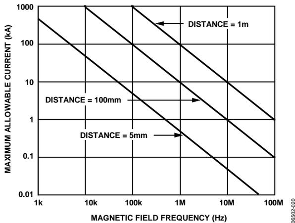
Figure 19. Maximum Allowable Current for Various Current-to-ADuM141x Spacings
