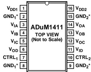
\*PIN 2 AND PIN 8 ARE INTERNALLY CONNECTED. CONNECTING BOTH TO GND<sub>1</sub> IS RECOMMENDED. PIN 9 AND PIN 15 ARE INTERNALLY CONNECTED. CONNECTING BOTH TO GND<sub>2</sub> IS RECOMMENDED.
