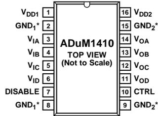
\*PIN 2 AND PIN 8 ARE INTERNALLY CONNECTED. CONNECTING BOTH TO GND<sub>1</sub> IS RECOMMENDED. PIN 9 AND PIN 15 ARE INTERNALLY CONNECTED. CONNECTING BOTH TO GND<sub>2</sub> IS RECOMMENDED.
