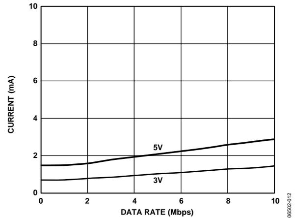
Figure 12. Typical ADuM1410 V<sub>DD2</sub> Supply Current vs. Data Rate for 5 V and 3 V Operation
