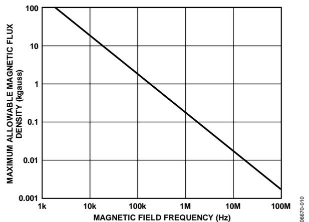
Figure 10. Maximum Allowable External Magnetic Flux Density
