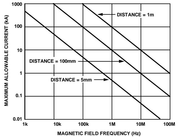
Figure 11. Maximum Allowable Current for Various Current-to-ADuM2250/ADuM2251 Spacings
