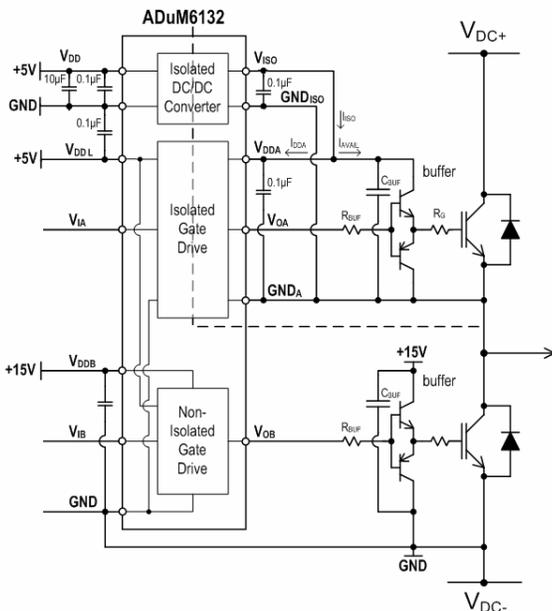
Figure 3. Typical Application Circuit
