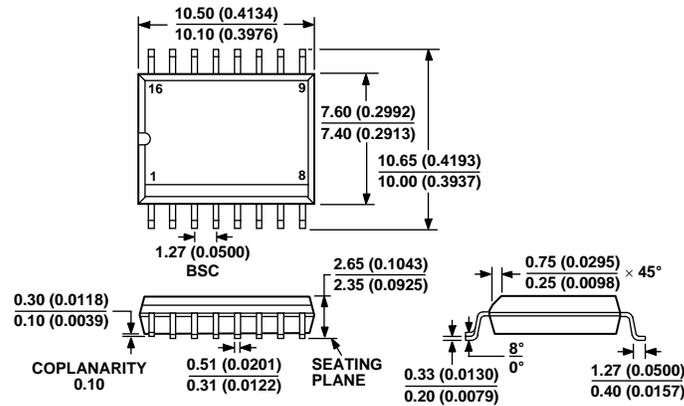
Figure 6. 16-Lead Standard Small Outline Package [SOIC]— Wide Body (RW-16).
