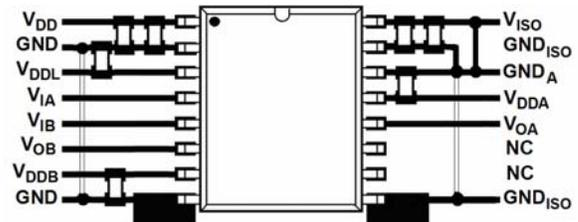
Figure 4. Recommended Printed Circuit Board Layout
