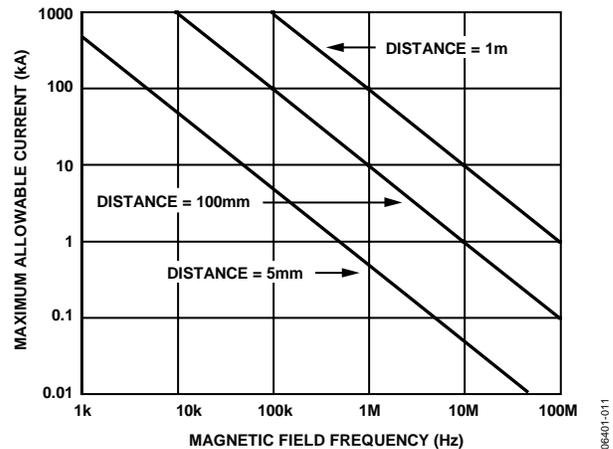
Figure 7. Maximum Allowable Current for Various Current-to-ADuM6132 Spacings
