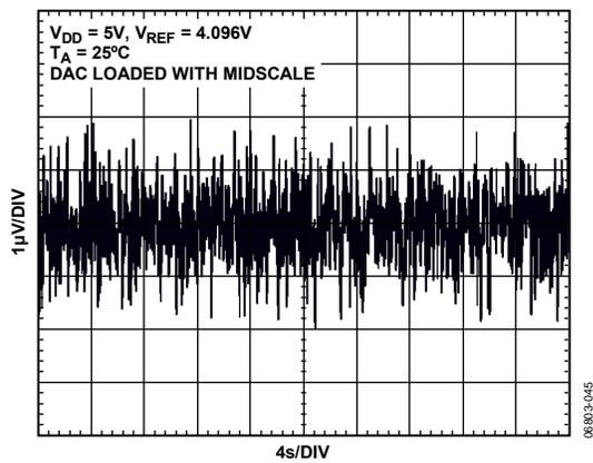
Figure 30. 0.1 Hz to 10 Hz Output Noise Plot
