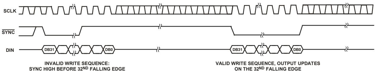
Figure 46.  $\overline{\text{SYNC}}$  Interrupt Facility
