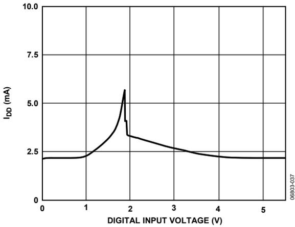
Figure 22. Supply Current vs. Digital Input Voltage
