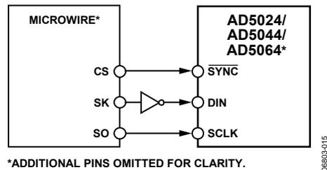
Figure 51. AD5024/AD5044/AD5064 to MICROWIRE Interface
