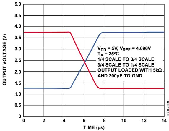
Figure 23. Settling Time
