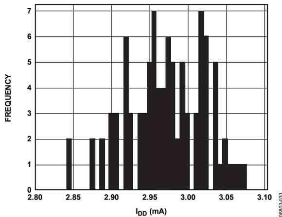
Figure 18.  $I_{DD}$  Histogram,  $V_{DD} = 5.0 V$
