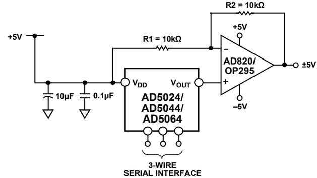
Figure 53. Bipolar Operation
