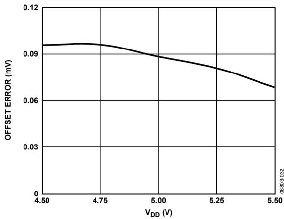
Figure 17. Offset Error Voltage vs. Supply Voltage
