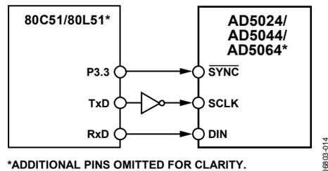
Figure 50. AD5024/AD5044/AD5064 to 80C51/80L51 Interface
