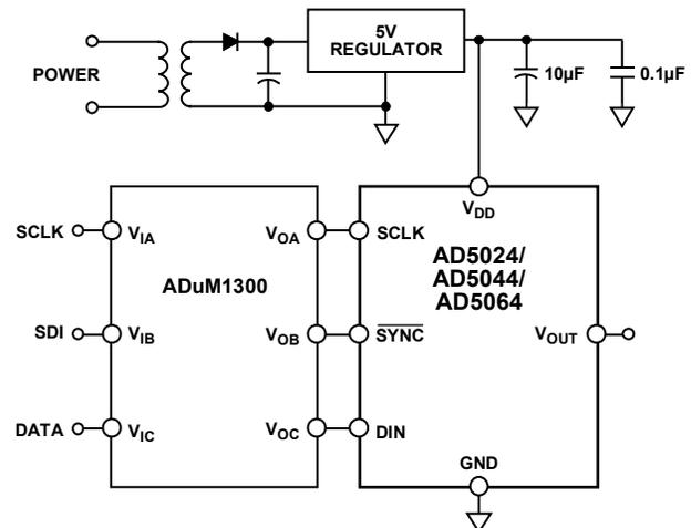
Figure 54. AD5024/AD5044/AD5064 with a Galvanically Isolated Interface
