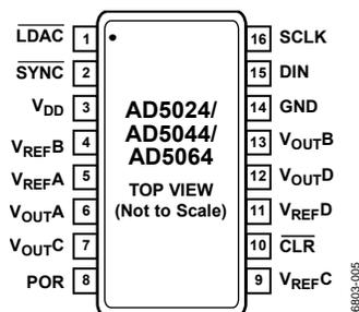
Figure 3. 16-Lead TSSOP (RU-16) Pin Configuration
