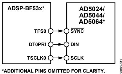
Figure 48. AD5024/AD5044/AD5064 to Blackfin ADSP-BF53x Interface
