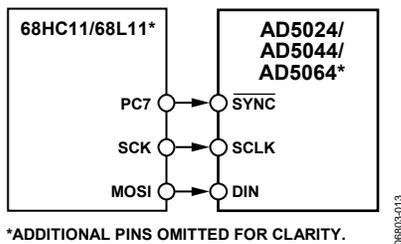
Figure 49. AD5024/AD5044/AD5064 to 68HC11/68L11 Interface
