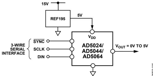
Figure 52. REF195 as Power Supply to the AD5024/AD5044/AD5064
