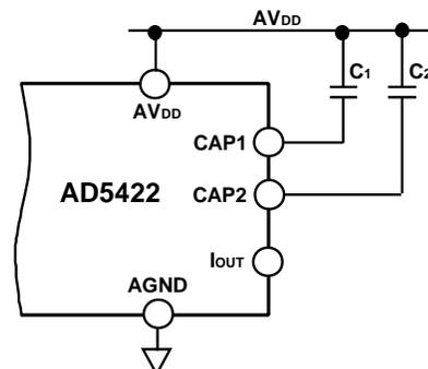
Figure 62. I<sub>OUT</sub> Filtering Capacitors
