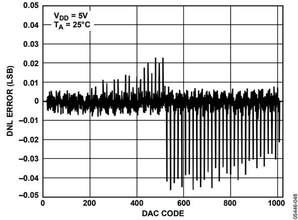
Figure 7. Typical AD5612 Differential Nonlinearity Error
