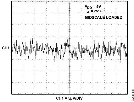
Figure 34. 1/f Noise, 0.1 Hz to 10 Hz Bandwidth
