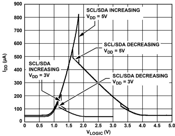
Figure 24. Supply Current vs. SCL/SDA Logic Voltage
