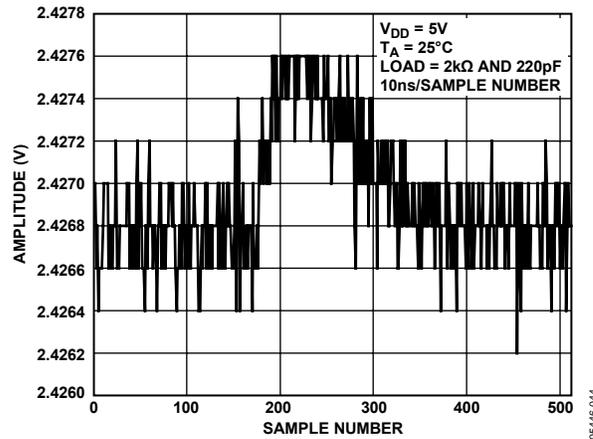
Figure 33. Digital Feedthrough
