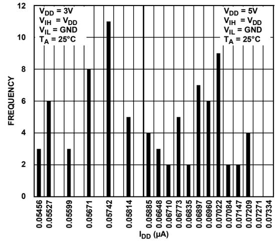
Figure 25.  $I_{DD}$  Histogram (3 V/5 V Supply)
