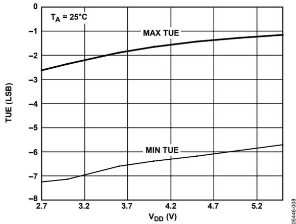
Figure 12. AD5622 Total Unadjusted Error vs. Supply
