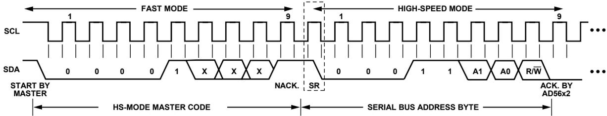
Figure 48. Placing the AD5602/AD5612/AD5622 into High Speed Mode
