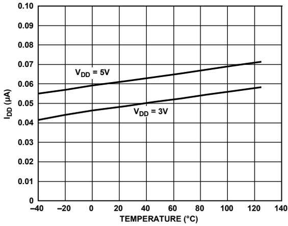
Figure 22. Supply Current vs. Temperature (3 V/5 V Supply)
