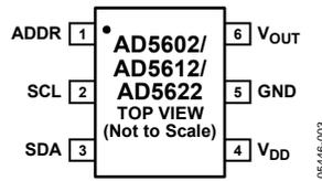
Figure 3. Pin Configuration
