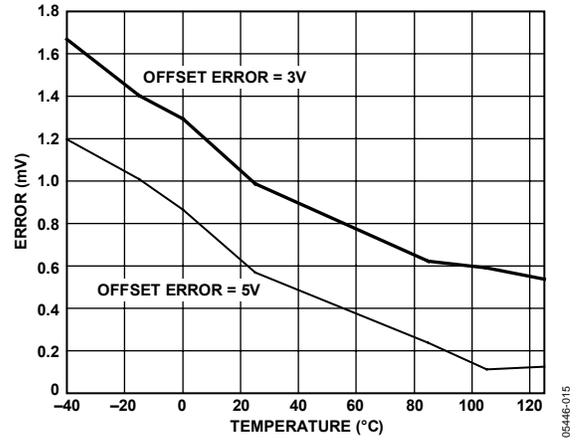
Figure 19. Offset Error vs. Temperature (3 V/5 V Supply)
