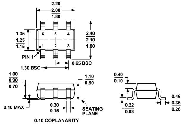
Figure 51. 6-Lead Thin Shrink Small Outline Transistor Package [SC70] (KS-6)
