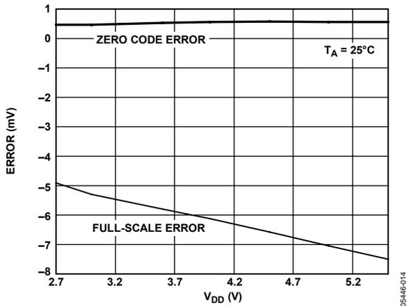
Figure 18. Zero Code/Full-Scale Error vs. Supply Voltage
