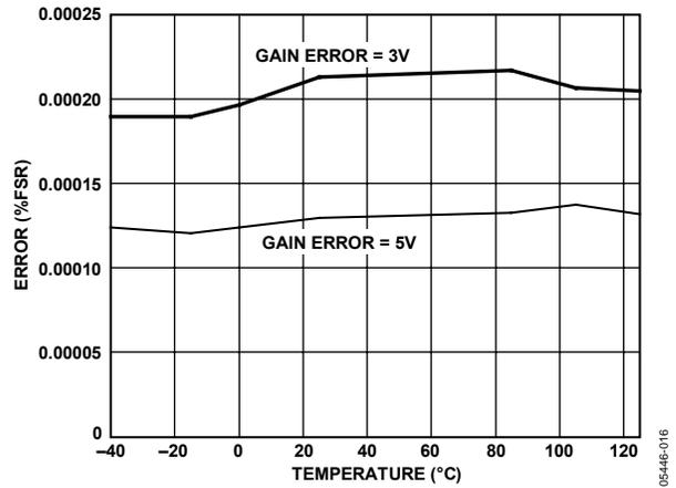
Figure 20. Gain Error vs. Temperature (3 V/5 V Supply)
