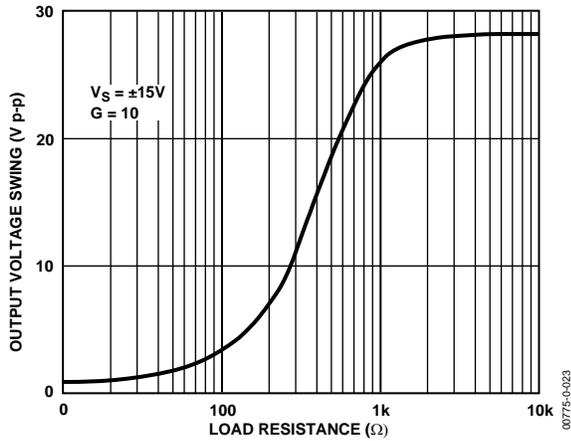
Figure 23. Output Voltage Swing vs. Load Resistance
