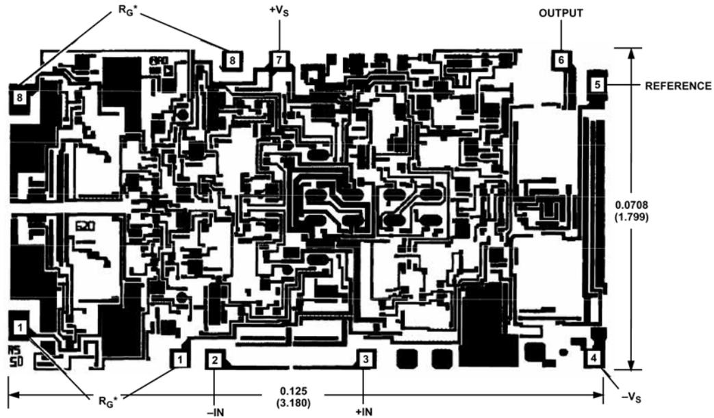
\*FOR CHIP APPLICATIONS: THE PADS  $1R_G$  AND  $8R_G$  MUST BE CONNECTED IN PARALLEL TO THE EXTERNAL GAIN REGISTER  $R_G$ . DO NOT CONNECT THEM IN SERIES TO  $R_G$ . FOR UNITY GAIN APPLICATIONS WHERE  $R_G$  IS NOT REQUIRED, THE PADS  $1R_G$  MAY SIMPLY BE BONDED TOGETHER, AS WELL AS THE PADS  $8R_G$ .
