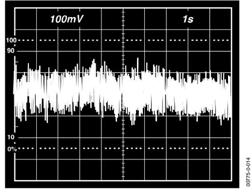
Figure 14. 0.1 Hz to 10 Hz Current Noise, 5 pA/Div
