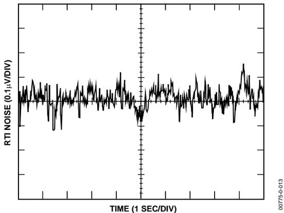
Figure 13. 0.1 Hz to 10 Hz RTI Voltage Noise ( $G = 1000$ )
