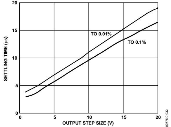
Figure 32. Settling Time vs. Step Size ( $G = 1$ )
