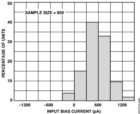
Figure 6. Typical Distribution of Input Bias Current
