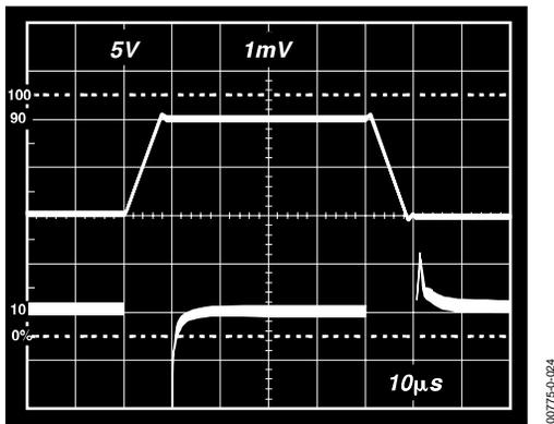
Figure 24. Large Signal Pulse Response and Settling Time
