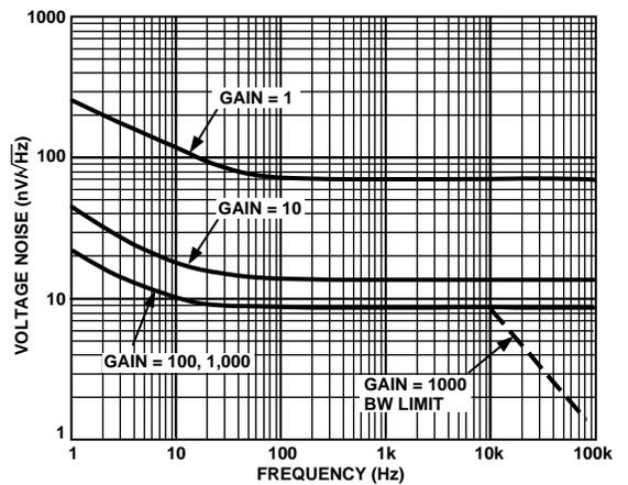
Figure 10. Voltage Noise Spectral Density vs. Frequency ( $G = 1-1000$ )
