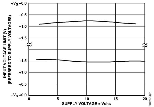
Figure 21. Input Voltage Range vs. Supply Voltage, G = 1
