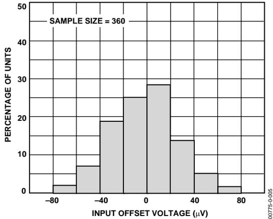
Figure 5. Typical Distribution of Input Offset Voltage
