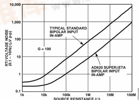
Figure 3. Total Voltage Noise vs. Source Resistance
