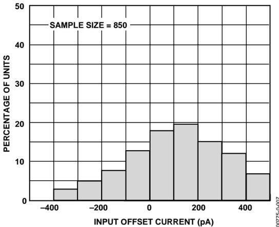
Figure 7. Typical Distribution of Input Offset Current
