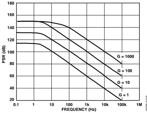
Figure 18. Negative PSR vs. Frequency, RTI (G = 1–1000)
