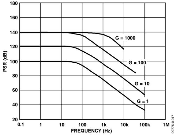
Figure 17. Positive PSR vs. Frequency, RTI (G = 1–1000)
