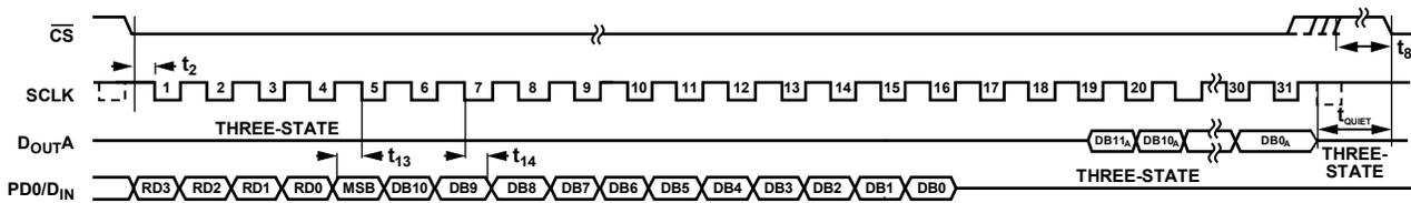
Figure 31. Timing Diagram for Writing to a Register
