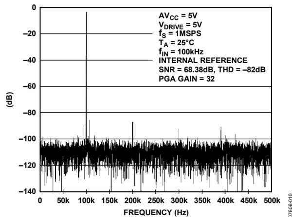
Figure 10. Typical FFT at Gain of 32
