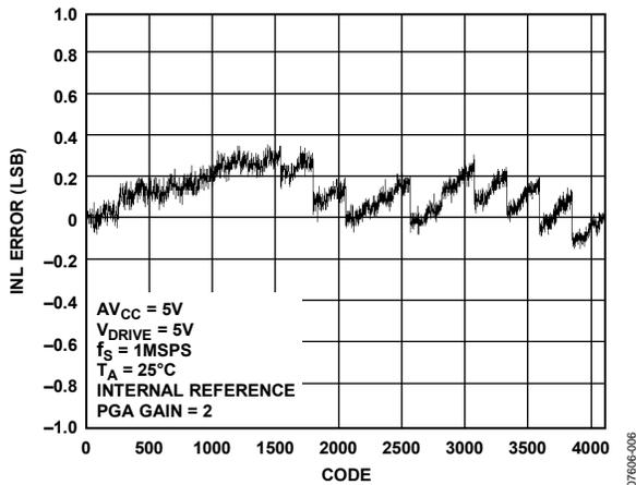
Figure 6. Typical INL at Gain of 2
