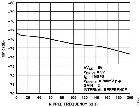
Figure 18. Common-Mode Rejection vs. Common-Mode Ripple Frequency
