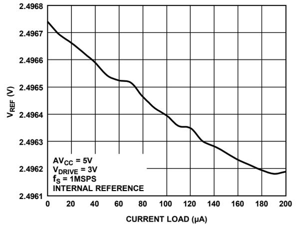
Figure 14.  $V_{REF}$  vs. Reference Output Current Load
