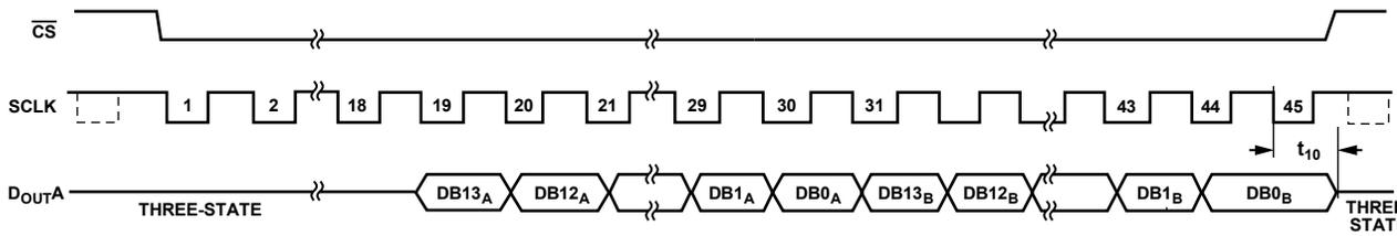
Figure 34. Reading Data from Both ADCs on One D<sub>OUT</sub> Line with 45 SCLKs
