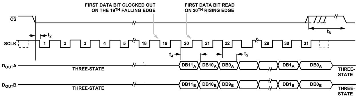
Figure 33. Serial Interface Timing Diagram When Reading Data on the 20<sup>th</sup> Rising SCLK Edge with a 40 MHz SCLK
