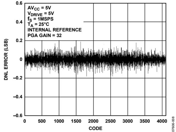
Figure 8. Typical DNL at Gain of 32
