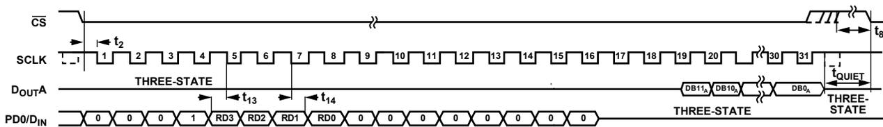
Figure 32. Timing Diagram for a Read Operation with PD0/D<sub>IN</sub> as an Input
