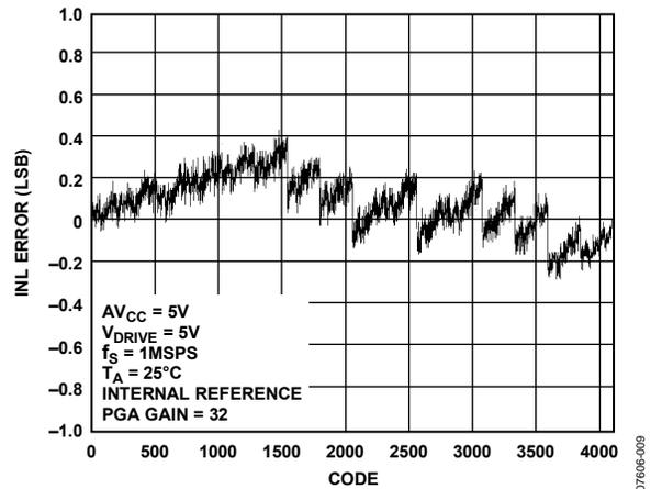
Figure 9. Typical INL at Gain of 32
