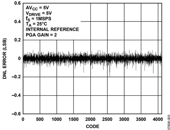
Figure 5. Typical DNL at Gain of 2
