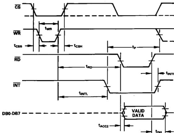
Figure 5a. WR-RD Mode ( $t_{RD} > t_{INTL}$ )
