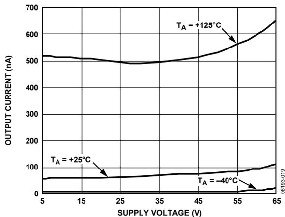
Figure 12. Output Current vs. Supply Voltage (Output Low)
