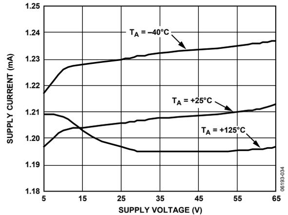
Figure 9. Supply Current vs. Supply Voltage (Output High)
