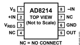
Figure 3. Pin Configuration
