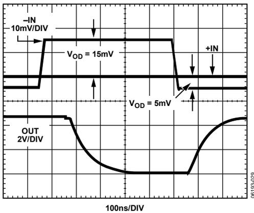
Figure 17. Typical Propagation Delay ( $R_{OUT} = 5\text{ k}\Omega$ )
