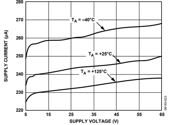
Figure 8. Supply Current vs. Supply Voltage (Output Low)
