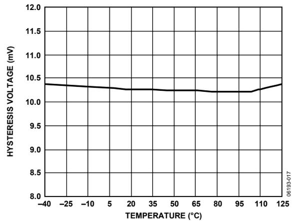
Figure 14. Hysteresis Voltage vs. Temperature ( $-IN$  Increasing)
