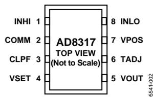
Figure 2. Pin Configuration
