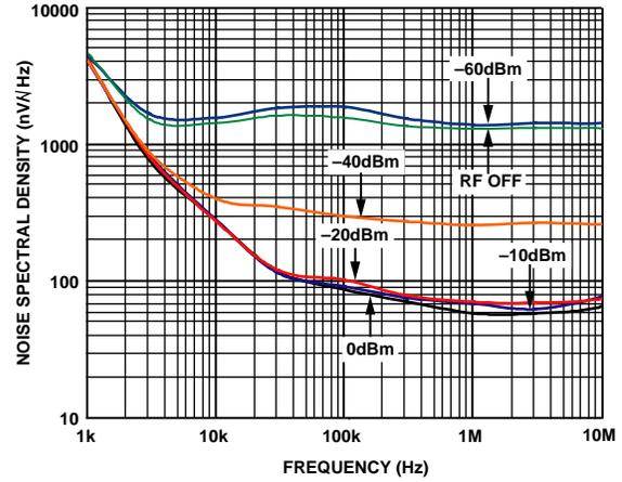
Figure 18. Noise Spectral Density of Output;  $C_{LPF} = \text{Open}$
