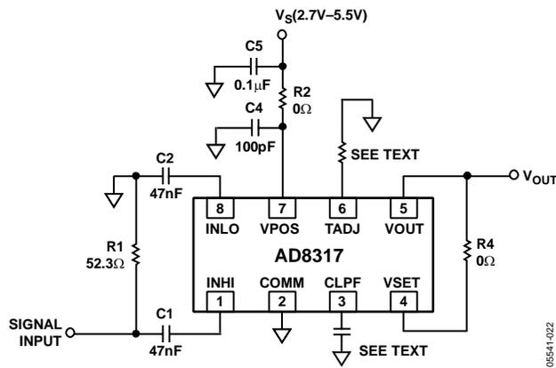
Figure 22. Basic Connections
