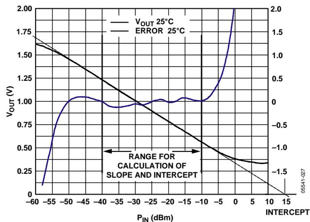
Figure 27. Typical Output Voltage vs. Input Signal
